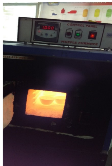
Calcination of raw fishbone
