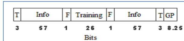
Figure2.6: GSM Normal Burst
