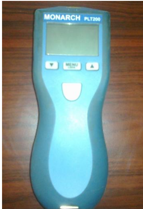
Figure 3.7b: Revolution speed measuring (MONARCH PLT200 type) tool used to measure speed of engine and generator (Source: Picture taken on site)
