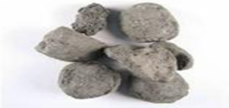
Figure 2.31: Typical burning in the kiln and clinker stones formation (Source: Operation manual)
