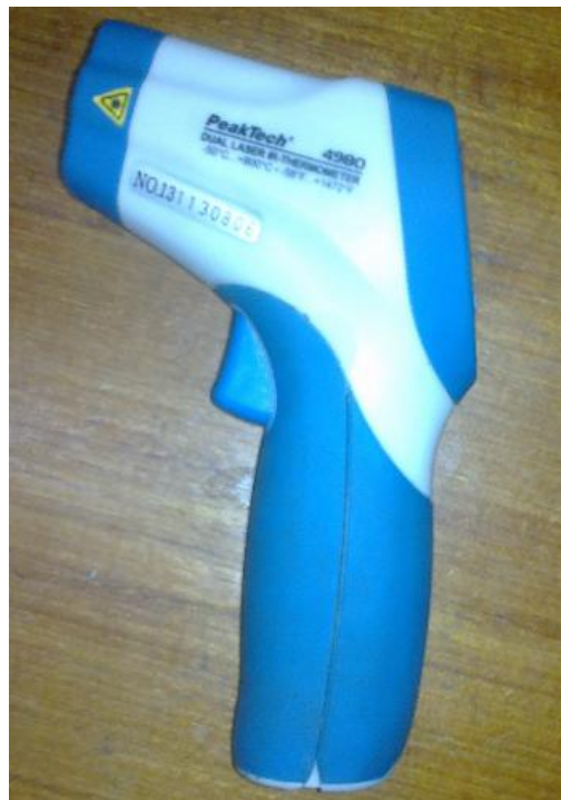
Figure 3.7a: Infrared thermometer (PeakTech 4980 type) used to measure ambient and coolant temperatures (Source: Picture taken on site)
