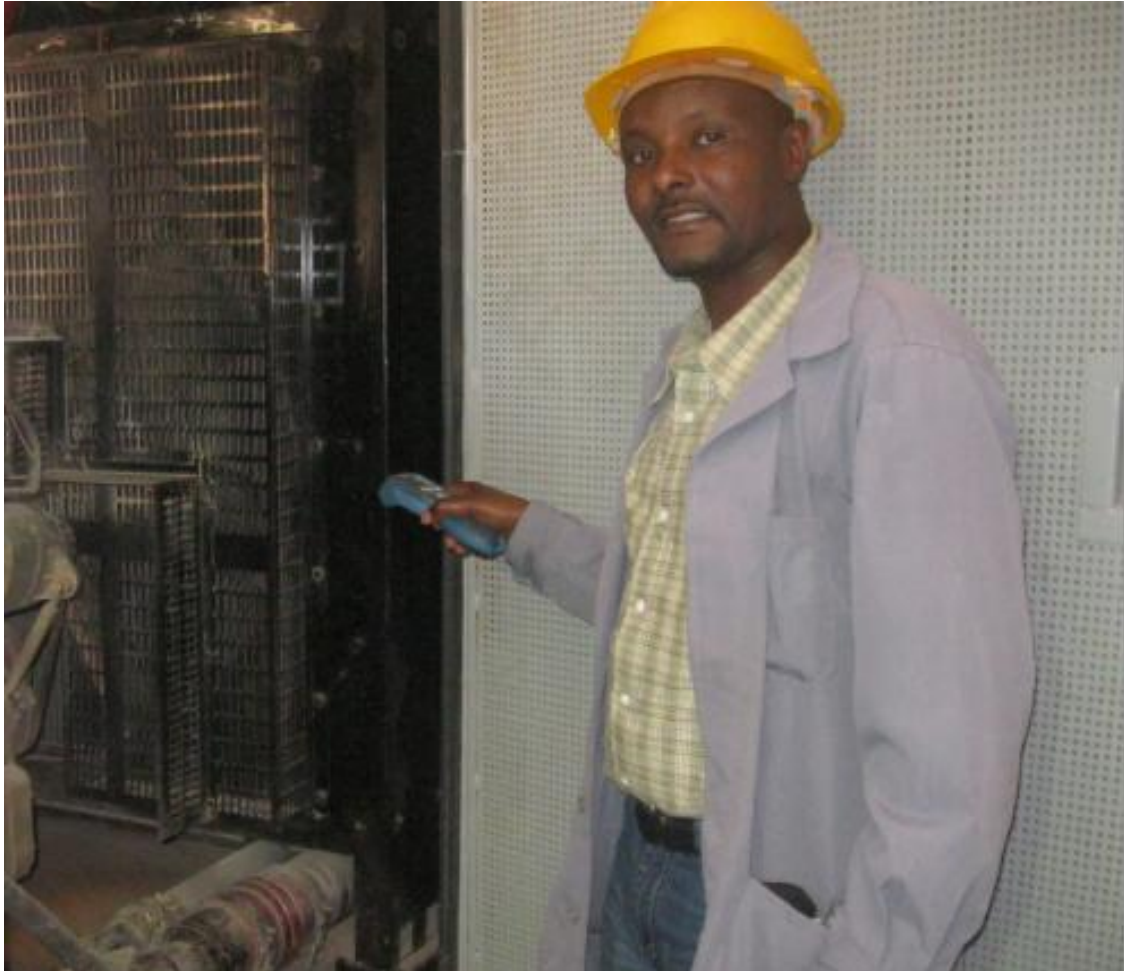
Figure 3.7d: Revolution speed measuring using (MONARCH PLT200 type) (Source: Picture taken on site)
