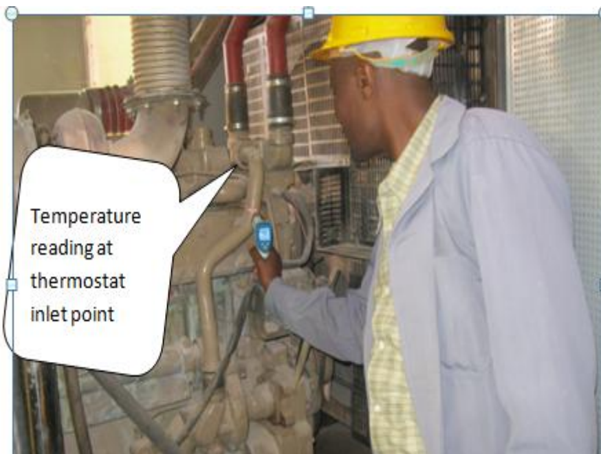
Figure 3.7c: Temperature measuring using PeakTech 4980 type infrared thermometer (Source: Picture taken on site)
