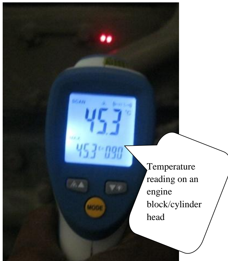
Figure 4.3: Temperature reading on an engine block/cylinder head (Source: Picture taken on site)
