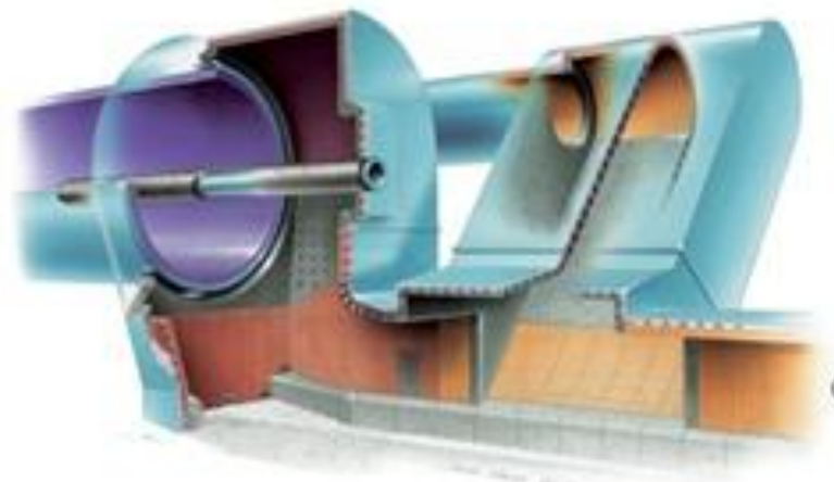
Figure 2.33: Clinker coolers (Source: Operation manual)
