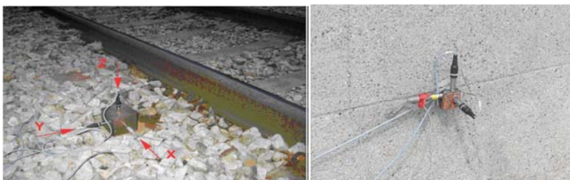
Figure 2-16 Measuring devices for vibrations [57]
