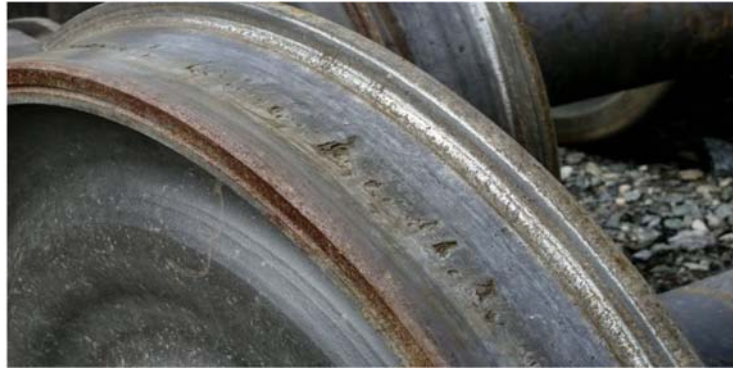
Figure 2-10 Wheel shelling defect [39]
