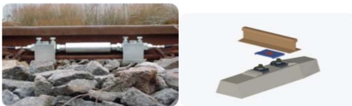
Figure 2-12 Laser and Strain gauge sensor [69]
