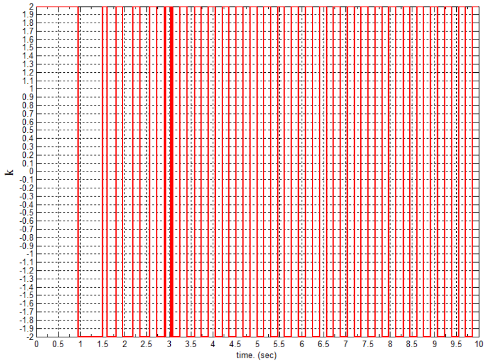
Figure 5.20: The variation of the switching gain with FSMC
