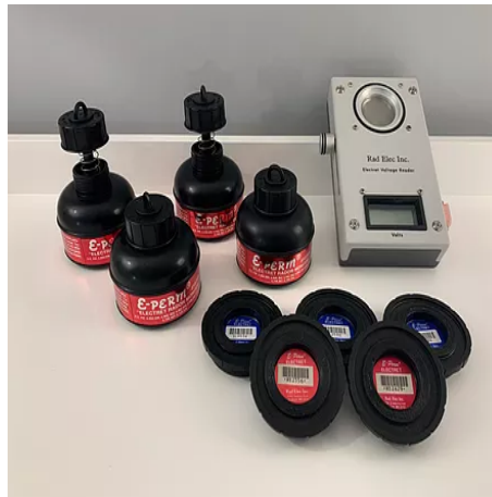
Figure 2.1: Electret ion chamber ( EIC )
