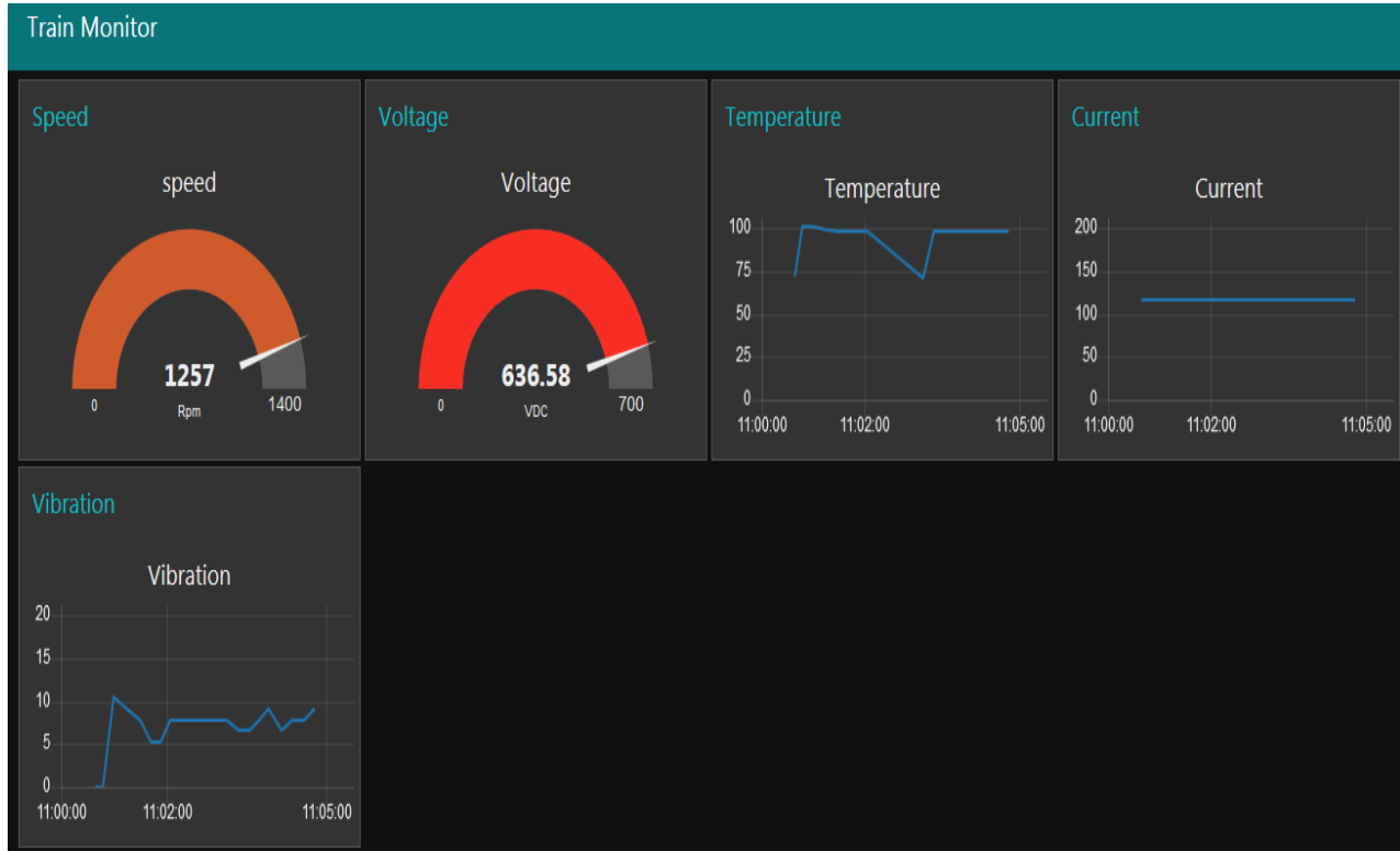
Figure 5-6: Figure showing sensor data being displayed on the dashboard in real-time.
