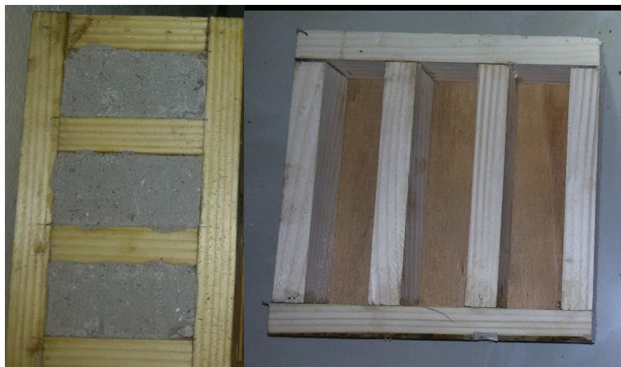
Figure 3.10 Compressive and flexural test specimens
