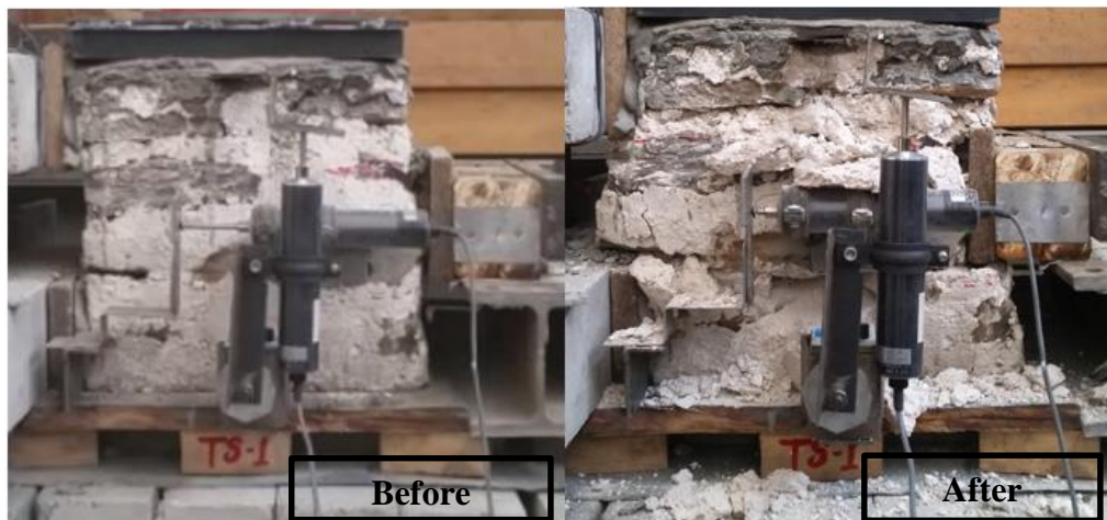
Figure 4.8 Failure mode of Specimen TS1
