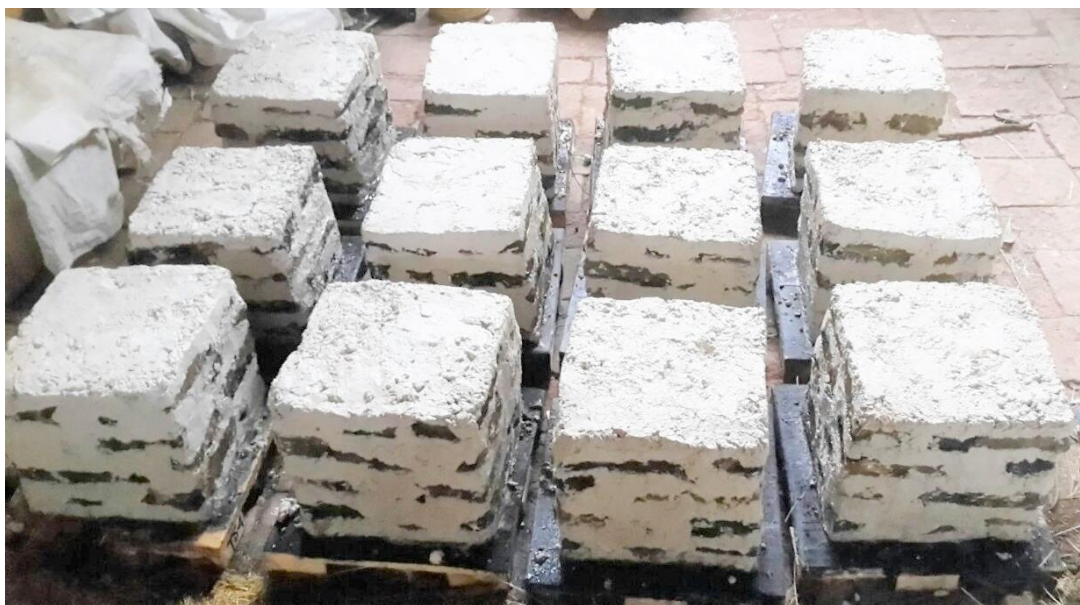
Figure 3.5 Masonry specimens during the curing period
