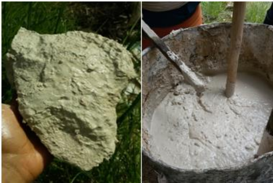
Figure 3.1 a) Hydrated lime unearthed from the slaking pit b) Hydrated lime agitated to form a lime putty
