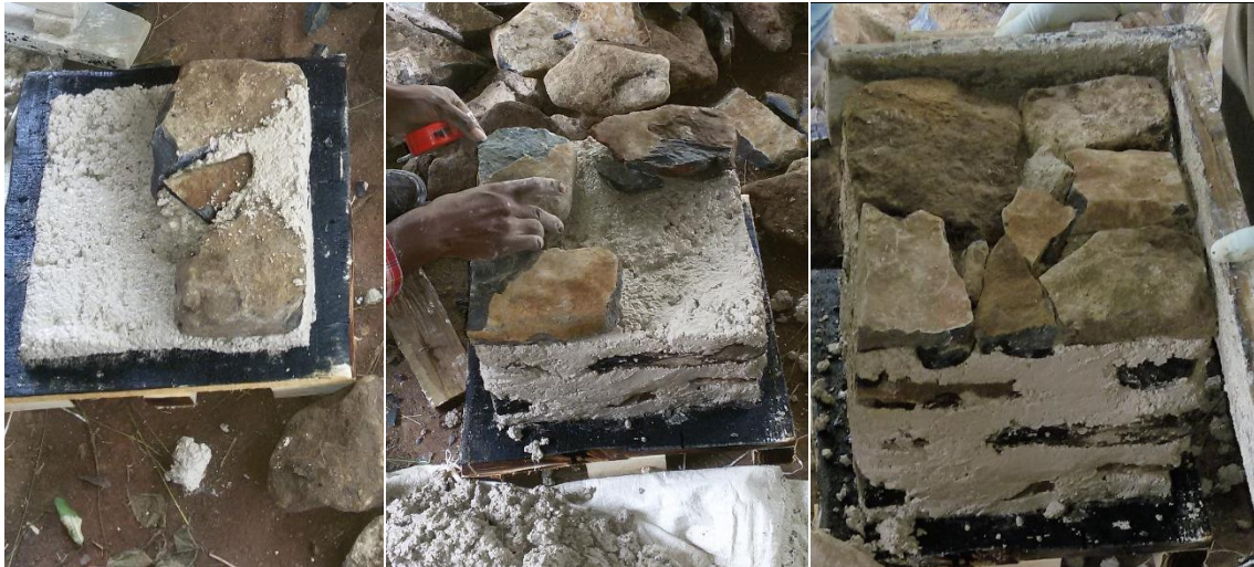
Figure 3.4 Masonry specimen construction
