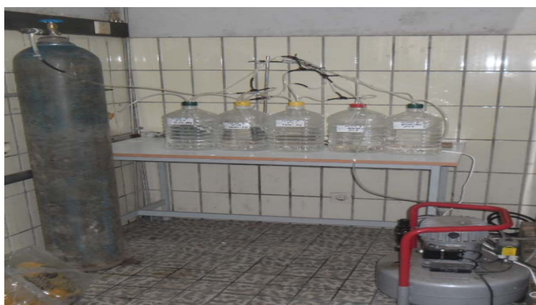
Figure 11. Laboratory set up for closed PBR culturing for determination of optimum algal biomass productivity (AAIT post graduate research lab)
