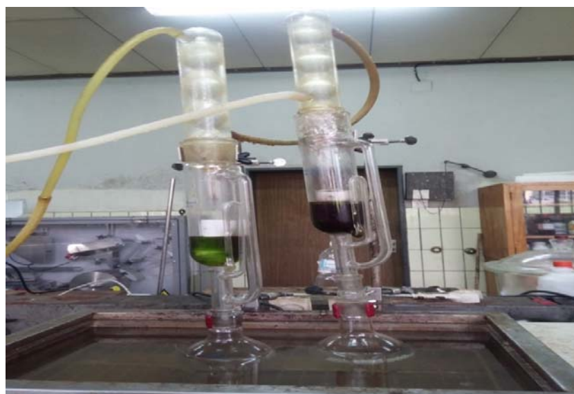
Figure 13 .Soxhlet extraction set up for extraction of algal oil
