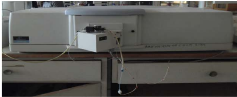
Figure 12. Perkin Elmer spectrophotometer for measurement of optical density of algal biomass at 515 nm.
