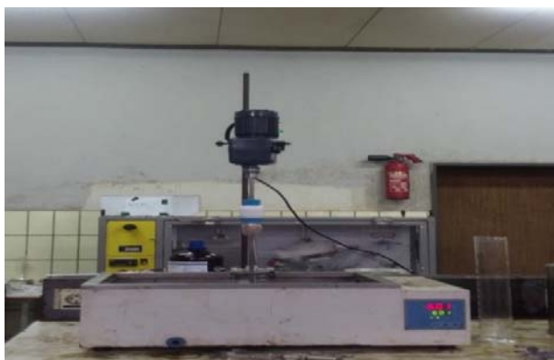
Figure 14. Transesterification of algal oil to biodiesel
