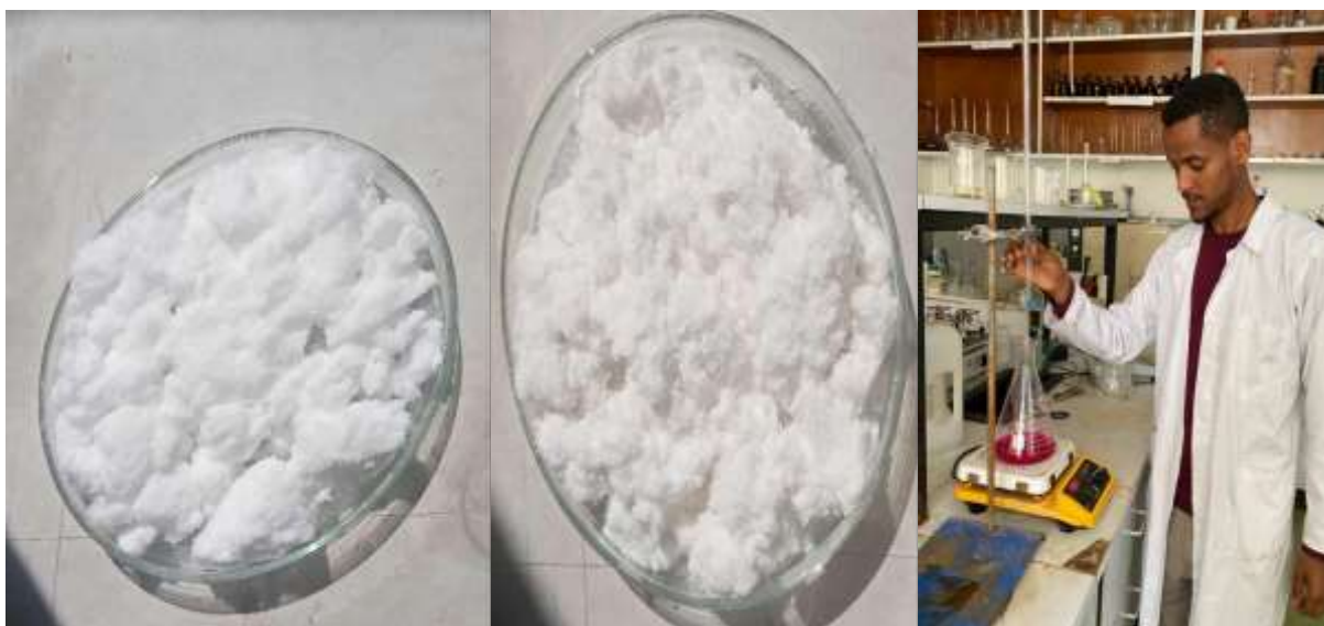
Figure 8: L-CMC (Carboxymethyl cellulose extracted from Phoenix dactylifera L tree leaf), LB-CMC (Carboxymethyl cellulose extracted from Phoenix dactylifera L Leaf base), and procedure for determination DS of CMC (from left to the right).
