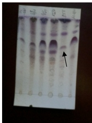
Figure 5.4. TLC bands of the extract from Streptomyces sp. Rv-355 shown in black arrow, the solvent system was a mixture of (Dichloromethane: Methanol 9:1, v/v)
