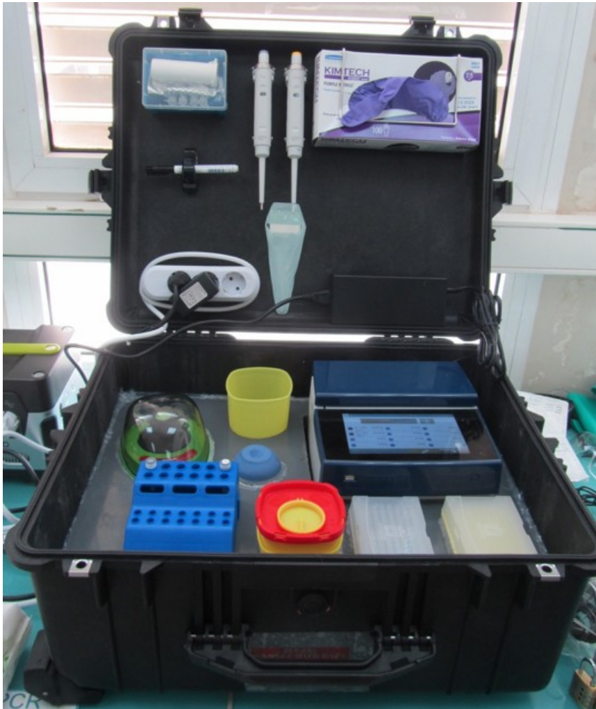
Figure 1 Mobile suitcase laboratory based on Recombinase Aided isothermal amplification assay accessories
