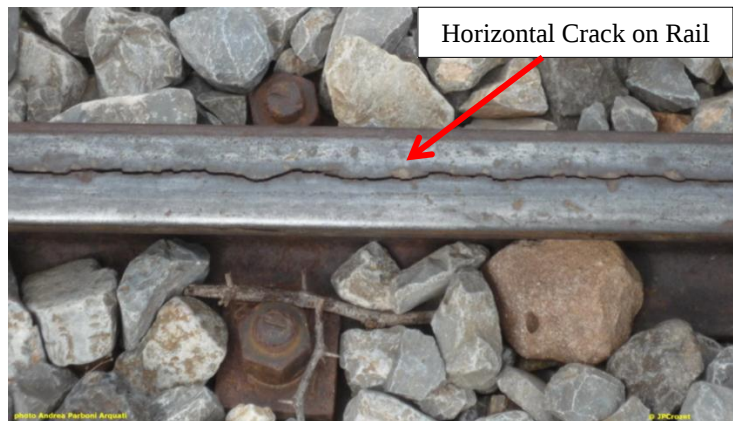
Vertical and Horizontal Crack on Rail, Ethio-Djibouti Railway Line 1964 [22]
