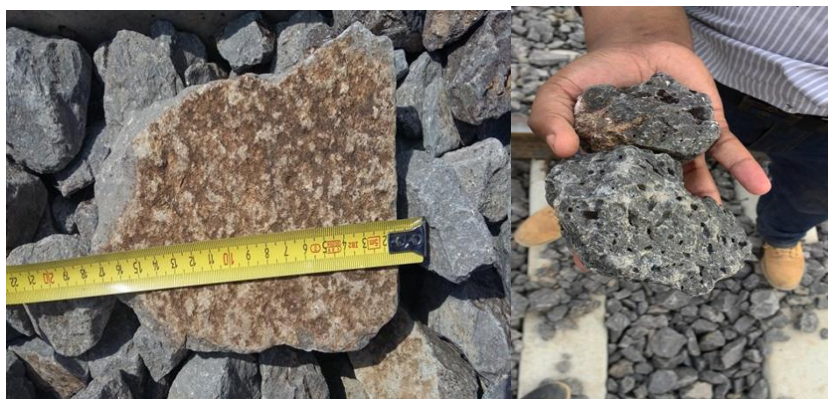
Oversized and Poor quality ballast respective along Adama-Awash Section [23]
