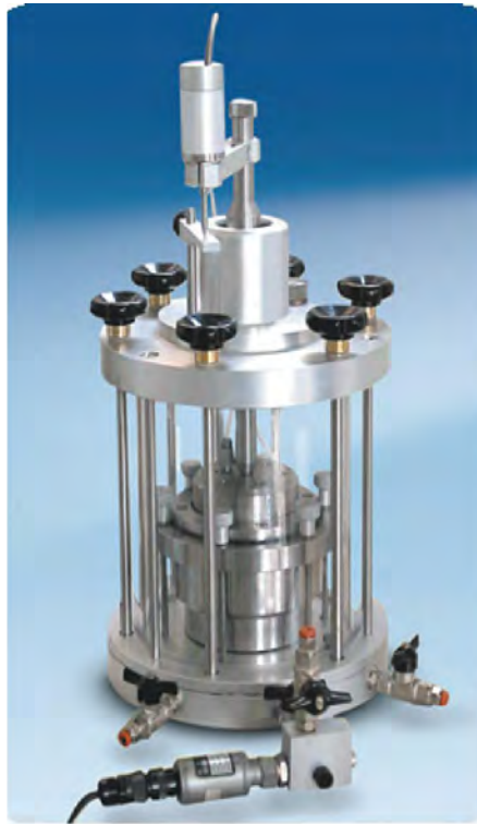
Fig.3.7: CRS consolidation cell [36].
