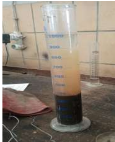
Figure 3.2 Silt content tests
