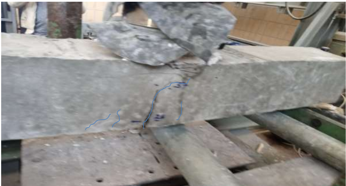
Figure 4.3 Flexural failure of specimen B23
