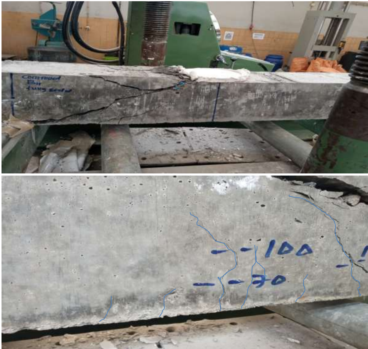
Figure 4.5 Flexural failure of specimen B11
