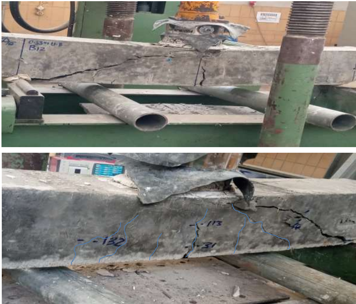
Figure 4.6 Flexural failure of specimen B12
