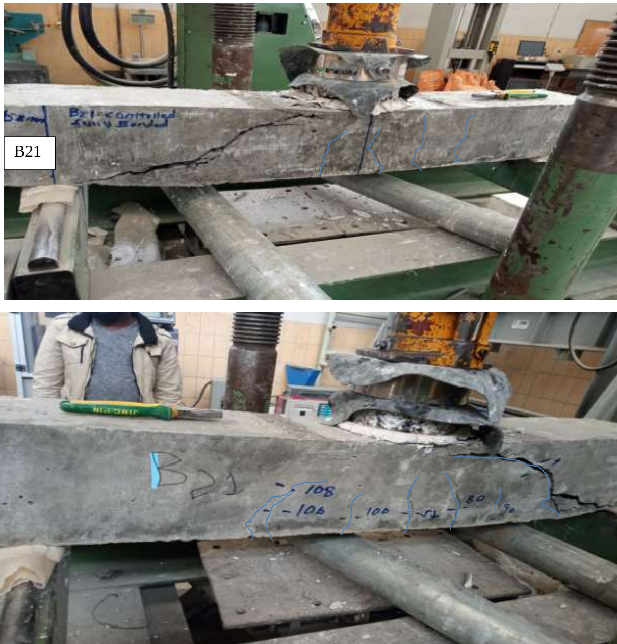
Figure 4.1 Flexural failure of specimen B21
