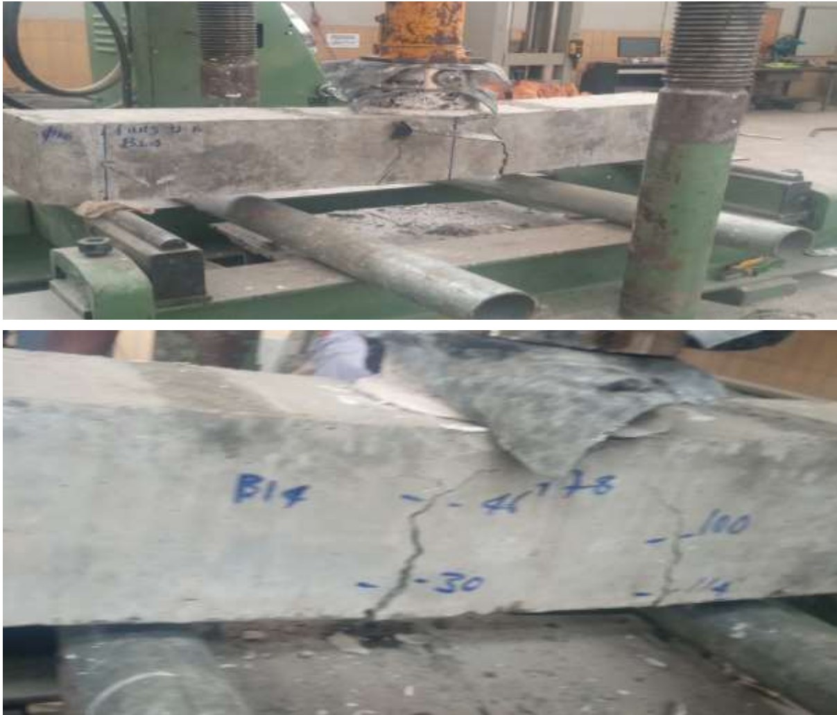
Figure 4.7 Flexural failure of specimen B14
