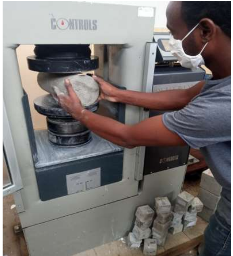
Figure 3.7 Tensile splitting tests:
