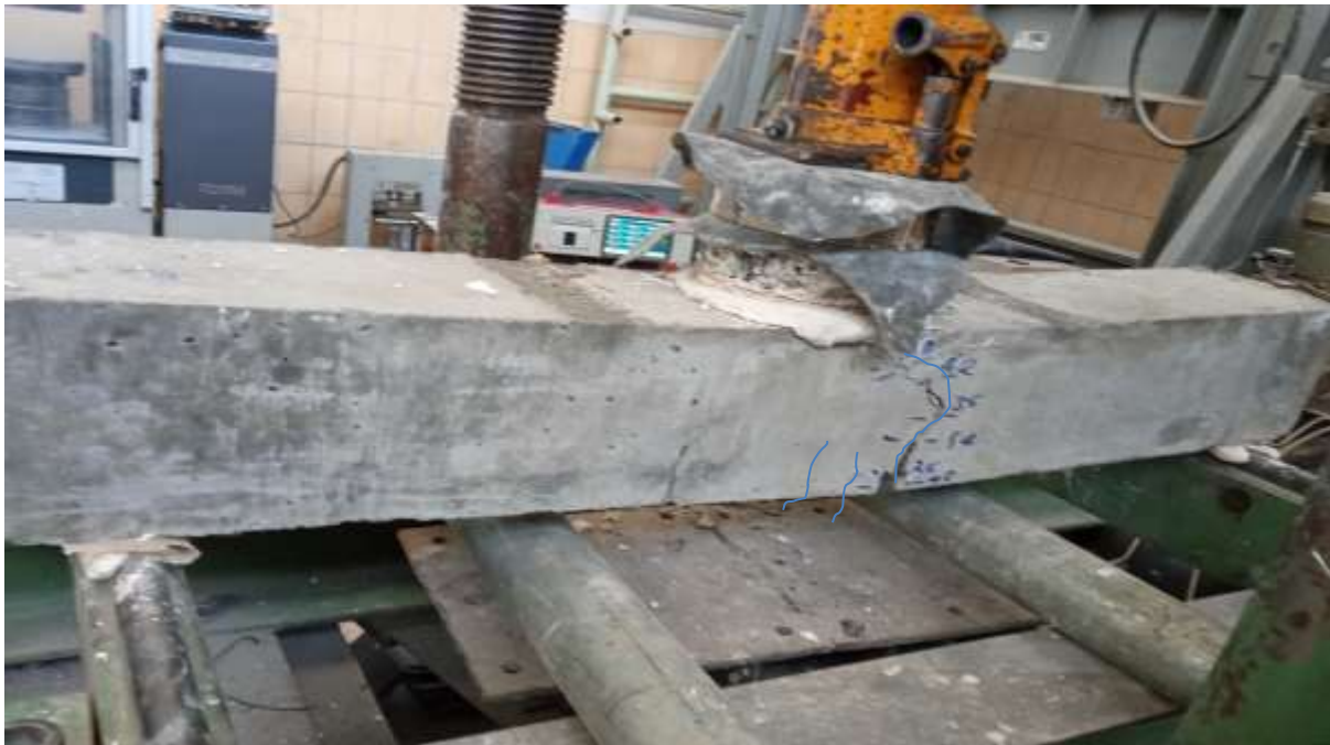
Figure 4.4 Flexural failure of specimen B24
