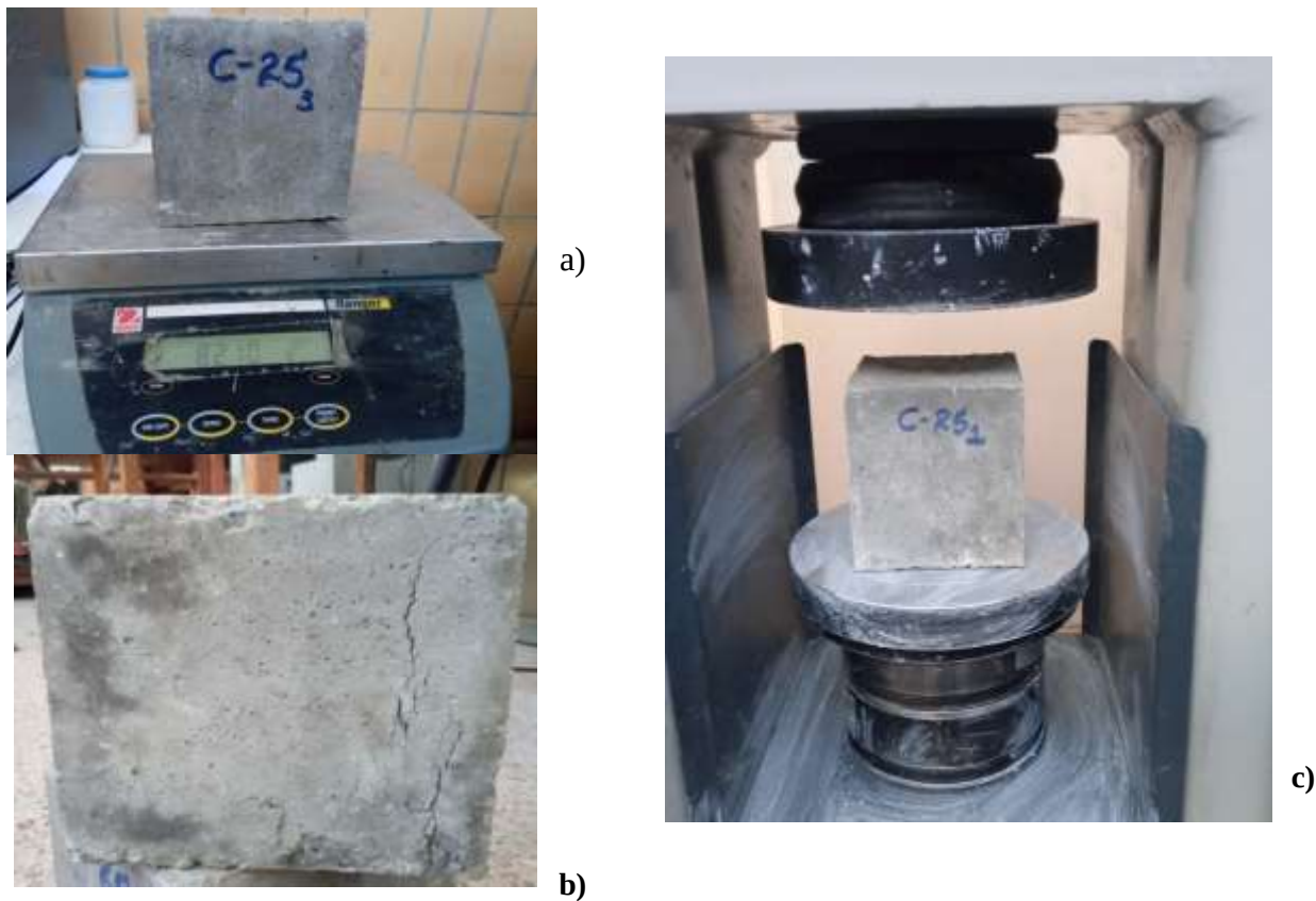
Figure 3.6 compressive strength tests: a) weighing b) Testing and c) crushed concrete after the test
