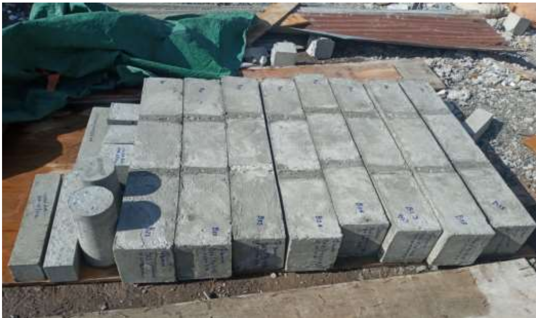
Figure 3.12 Beams casted outside laboratory
