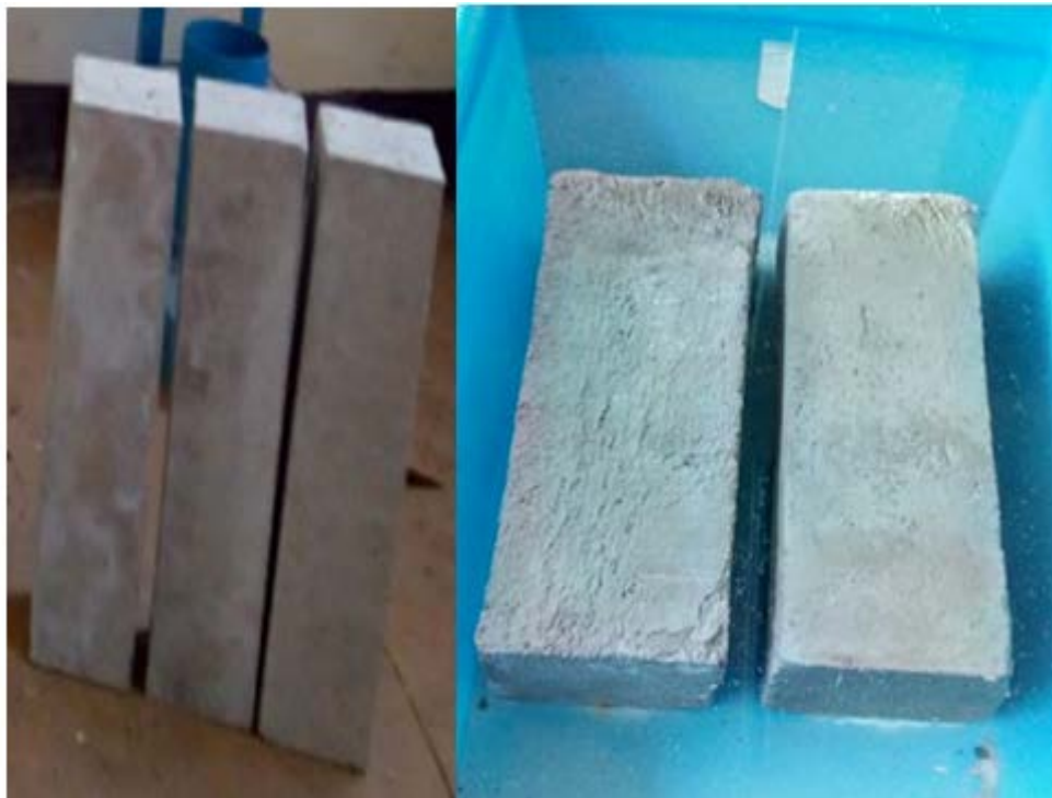
Figure 3-9: The Specimens of controls and Reinforced concrete strengthened by Ferro cement
