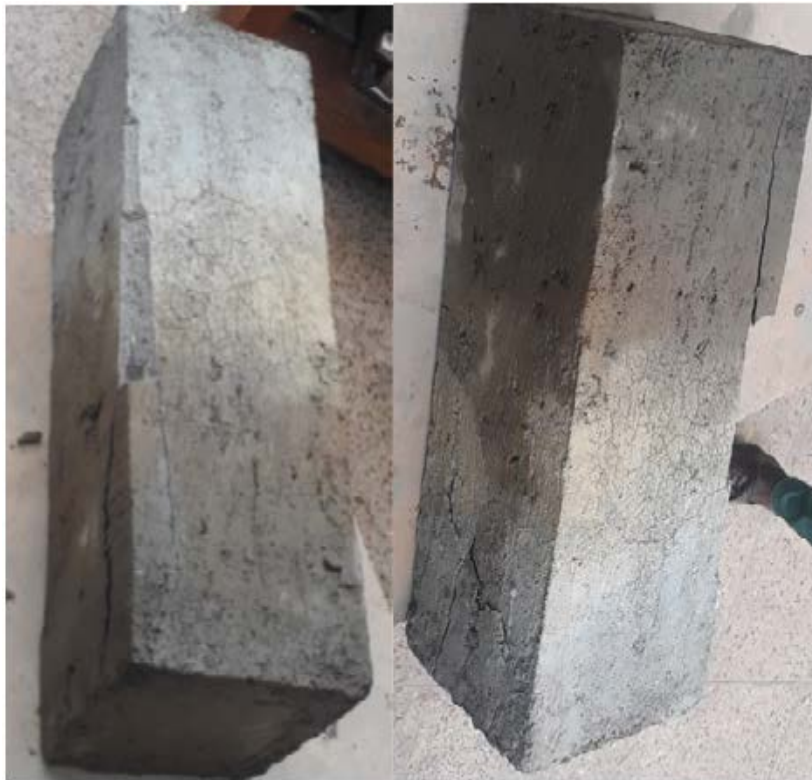
Figure 5-8: Typical failure pattern for MWCS
