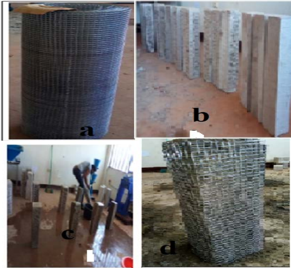
Figure 3-11: Preparation for strengthening : (a) Measuring, Cutting (b) chiseled specimen to create rough surface (c) put “buhaka” thin mix cement with water (d) mash wire and Put the square mesh on
