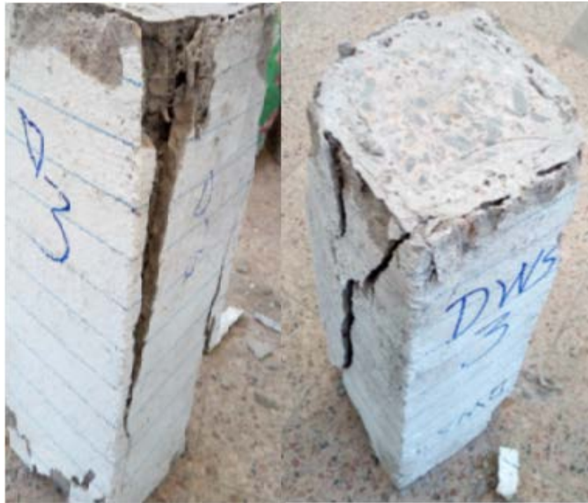
Figure 5-11: Typical failure pattern DWCS
