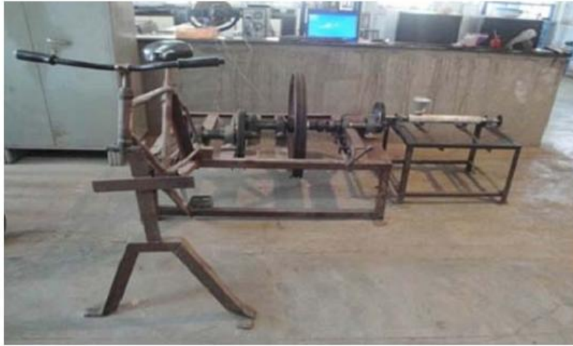
Fig.5 Oil press using human powered flywheel motor
