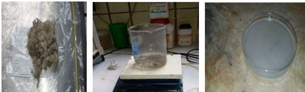
Figure 3.2: Preparation of glue: Collagen Hydrolysate, CH and water being boiled and final glue solution respectively
