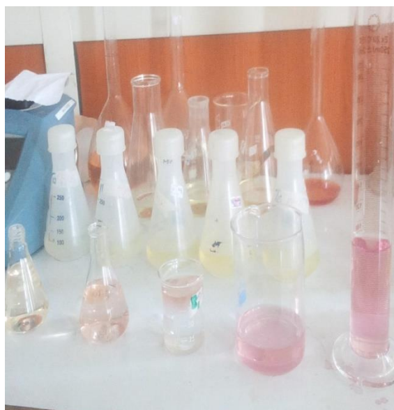
Cr (VI), 1,5-Diphenylcarbazine complex after adsorption
