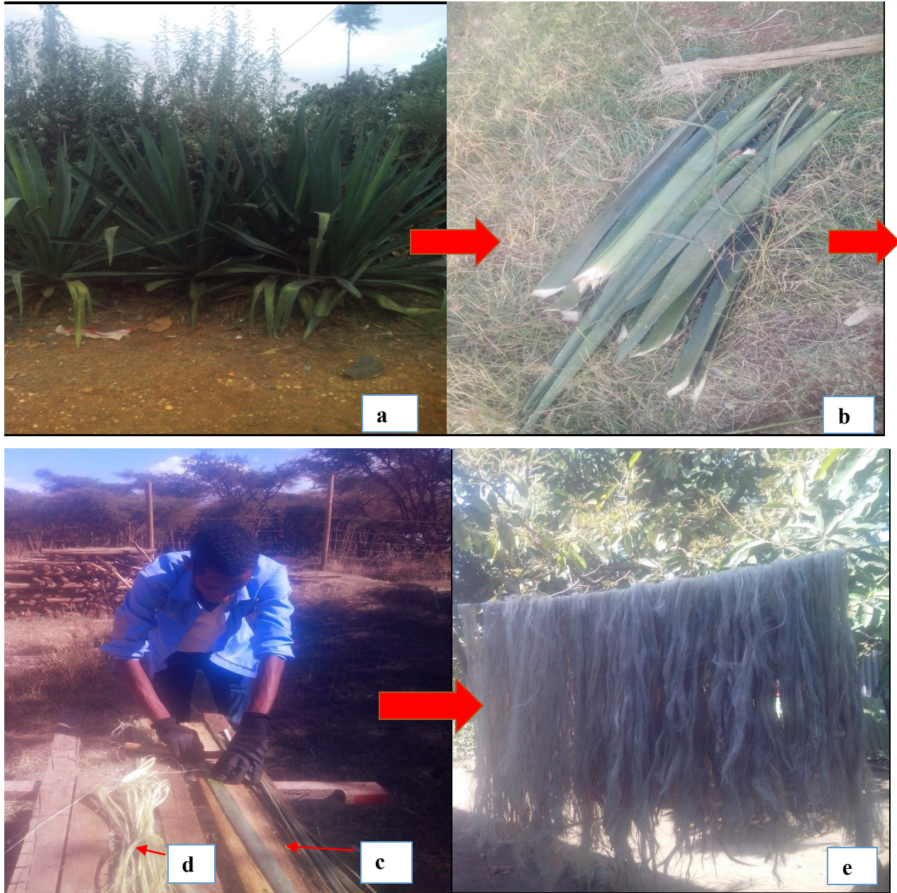
Figure 3.1. Manual extraction process of sisal fiber.
