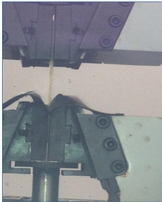
Figure 3.12. Typical tensile specimen under tensile test.
