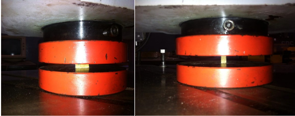
Figure 3.13. Typical specimens under transverse and longitudinal compression test.
