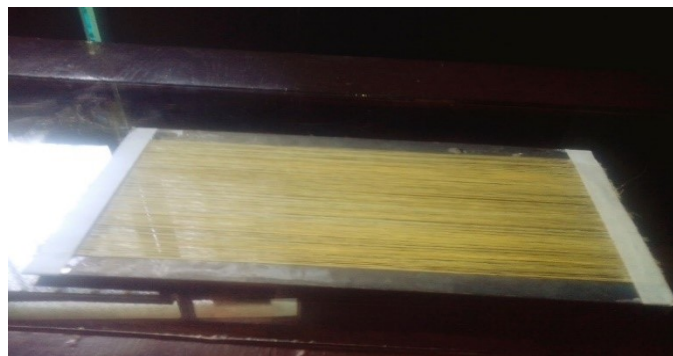
Figure 3.4. Unidirectional sisal fiber with frame
