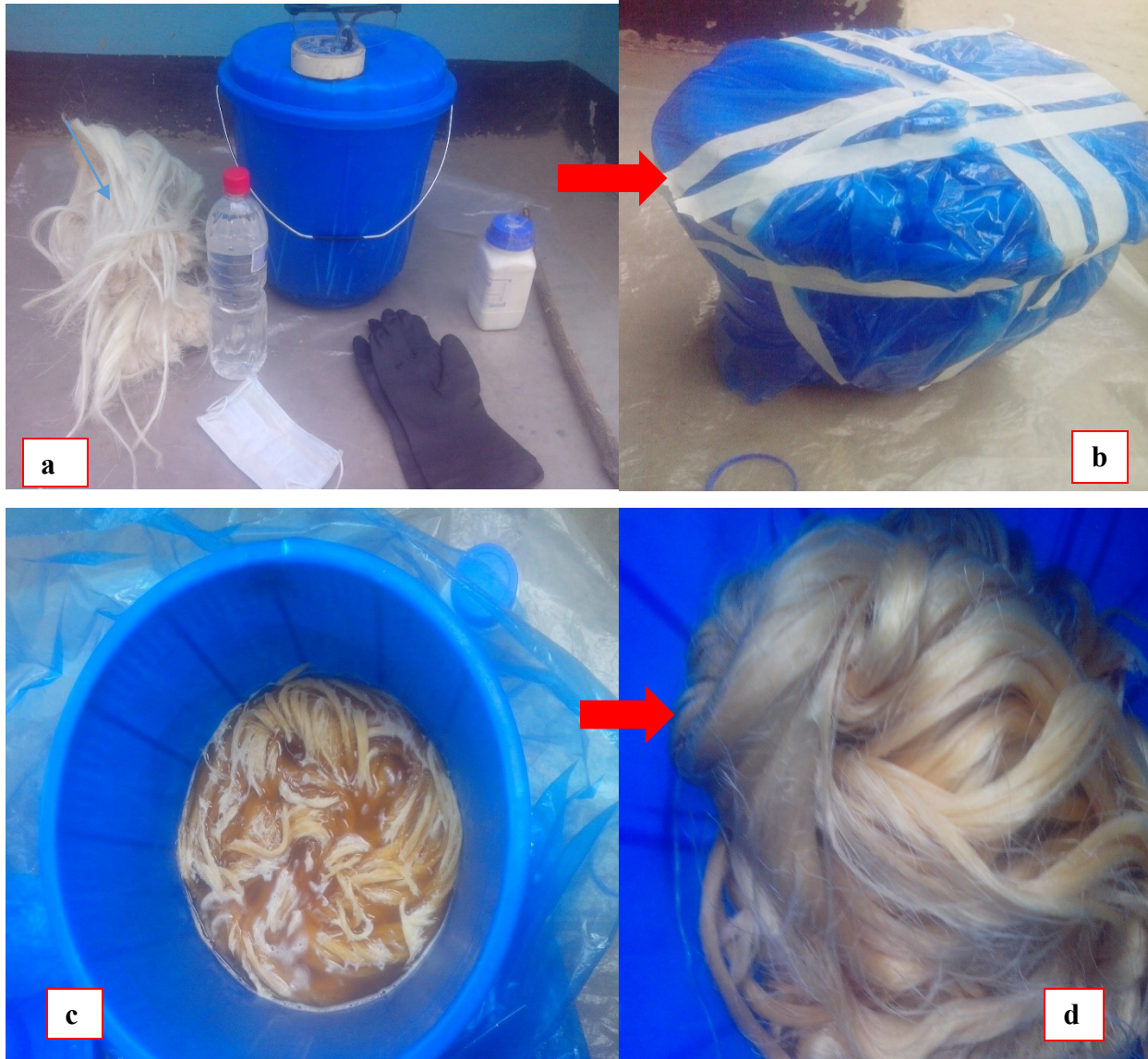
Figure 3.3. Alkaline treatment of sisal fiber.
