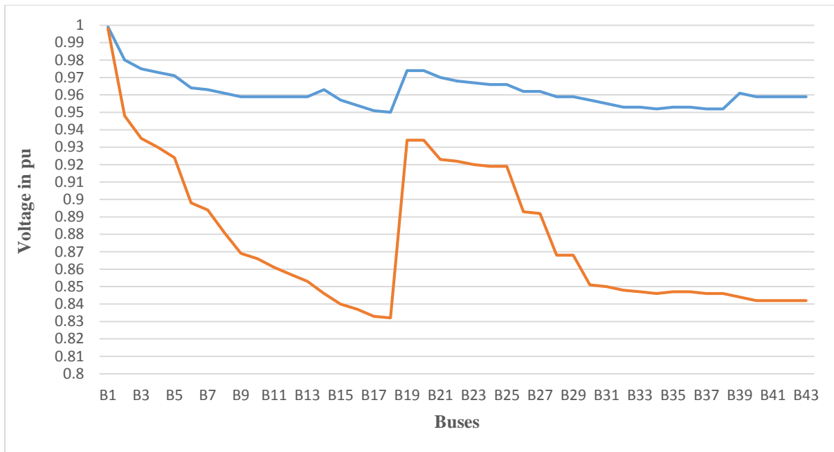
Figure 4. 19 Comparison of voltage profile of SEB-12 of Sebeta-I substation before and after DG integration
