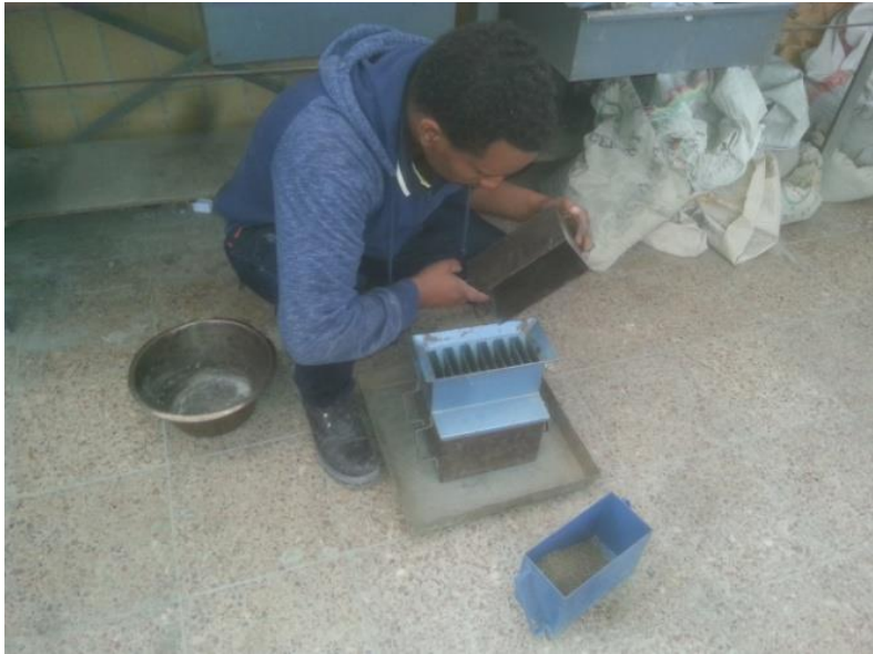
F-1 Dividing the sand into two part using riffler
