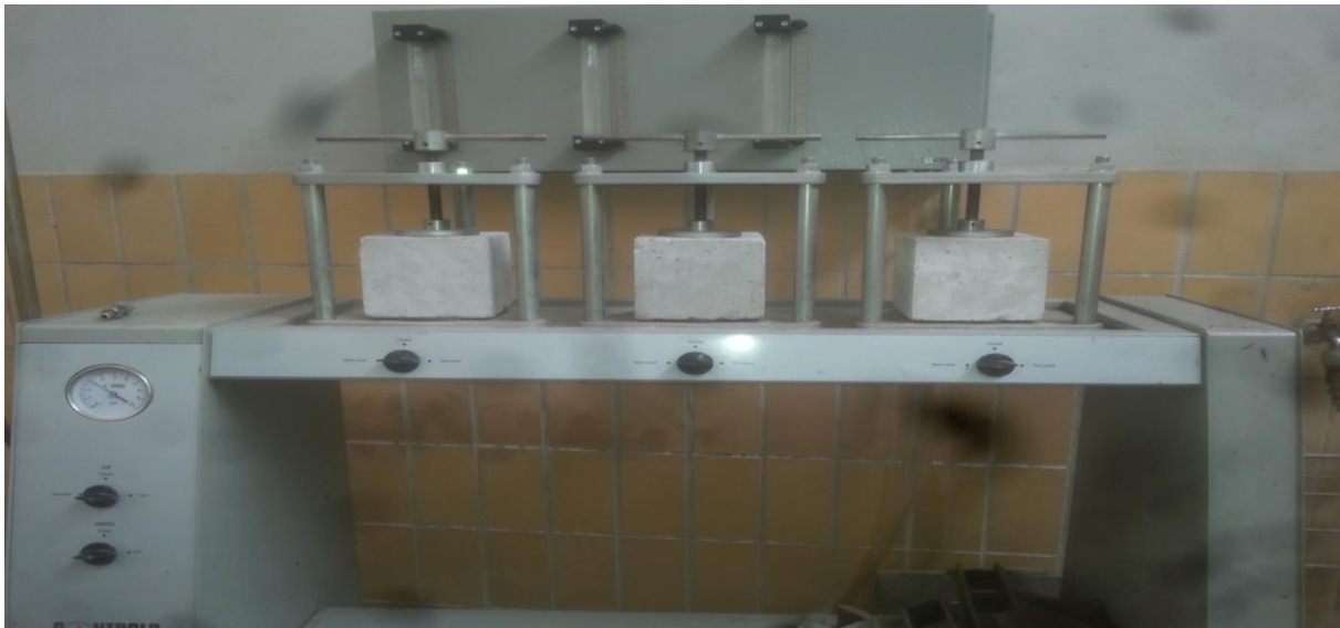
F-9 Concrete on Water permeability testing apparatus
