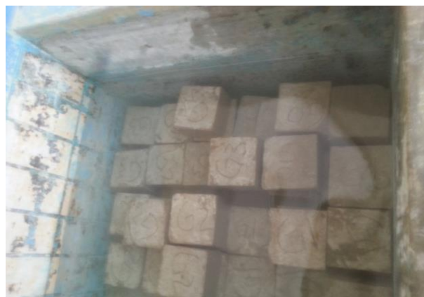
F-6 Concrete specimens after casting
