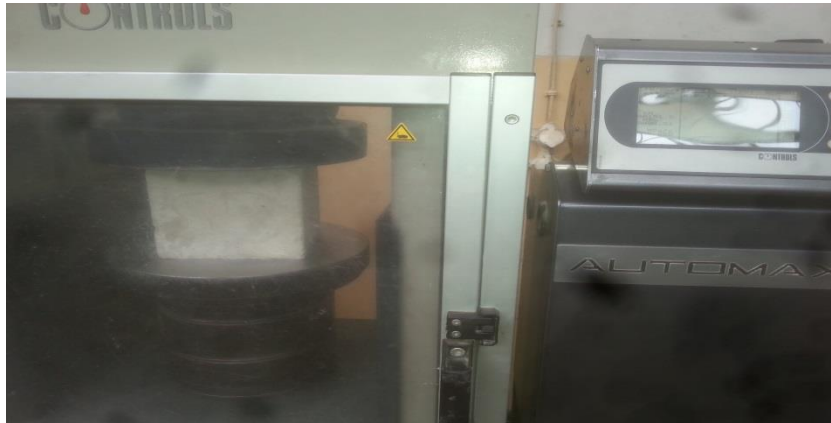
F-8 Concrete inside compression machine
