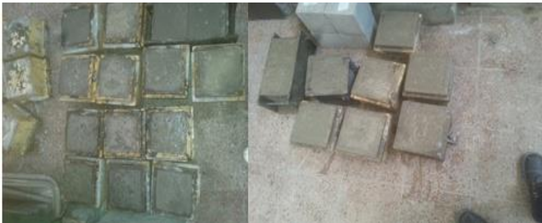
F-6 Concrete specimens after casting
