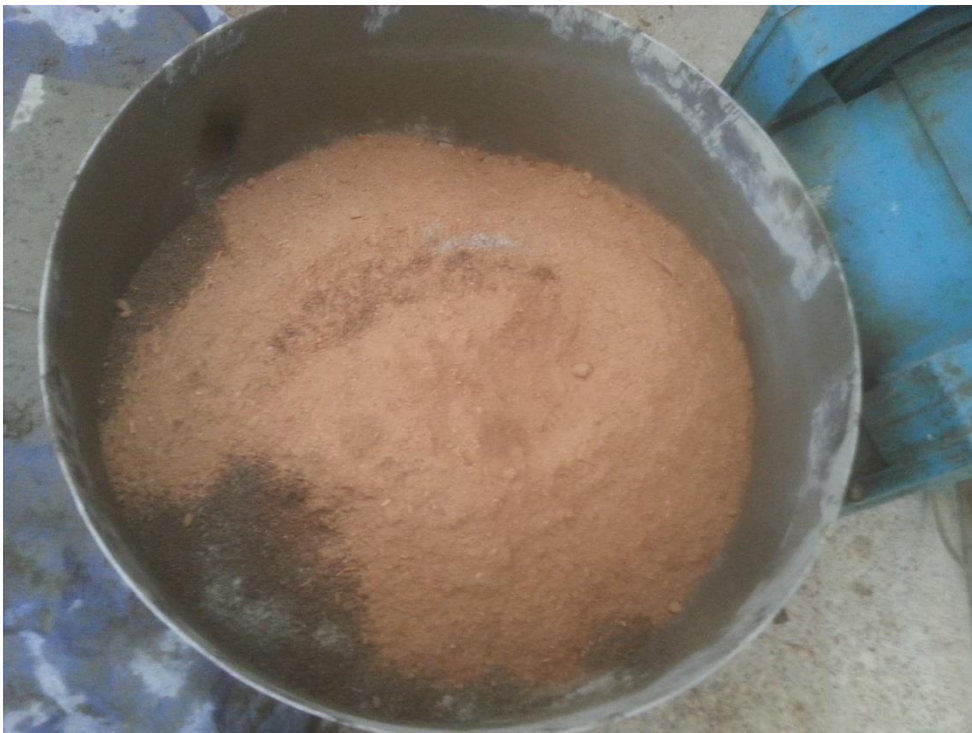
F-4 Sawdust inside the mixer
