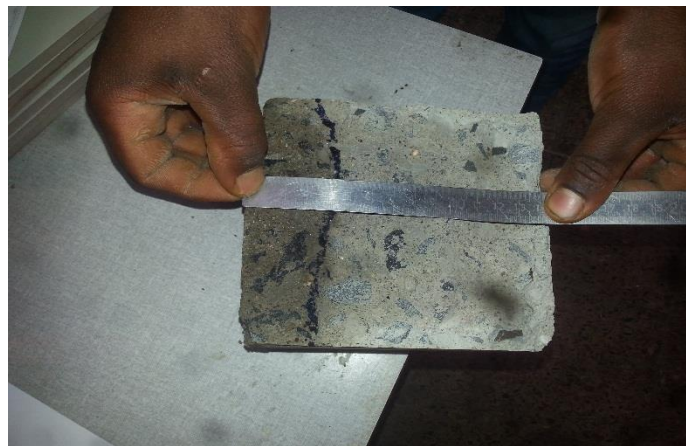
F-10 Measuring water penetration depth of the concrete
