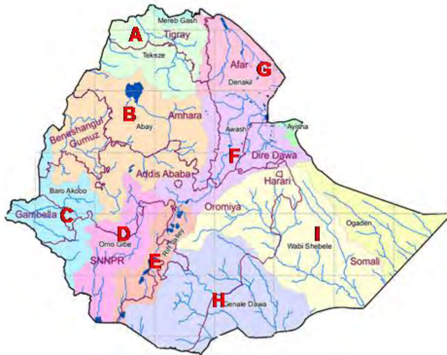
Figure 1. The drainage basins of Ethiopia (After UN-OCHA, 2006); A = Tekeze-Atbara, B = Abay (Blue Nile), C = Baro-Akobo (White Nile), D = Omo-Gibe (Omo-Turkana), E = Rift Valley lakes, F = Awash River, G = Danakil Depression, H = Genale-Dawa, I = Wabishebele
