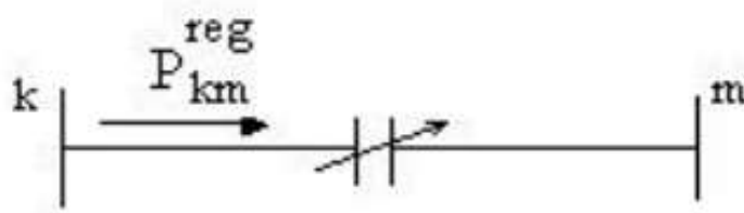
Figure 3.3: TCSC equivalent capacitive reactance [15]
