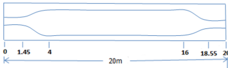
Figure 4.1: Points for the length of varying cross-section along the 20m simply supported post-tensioned box-girder
