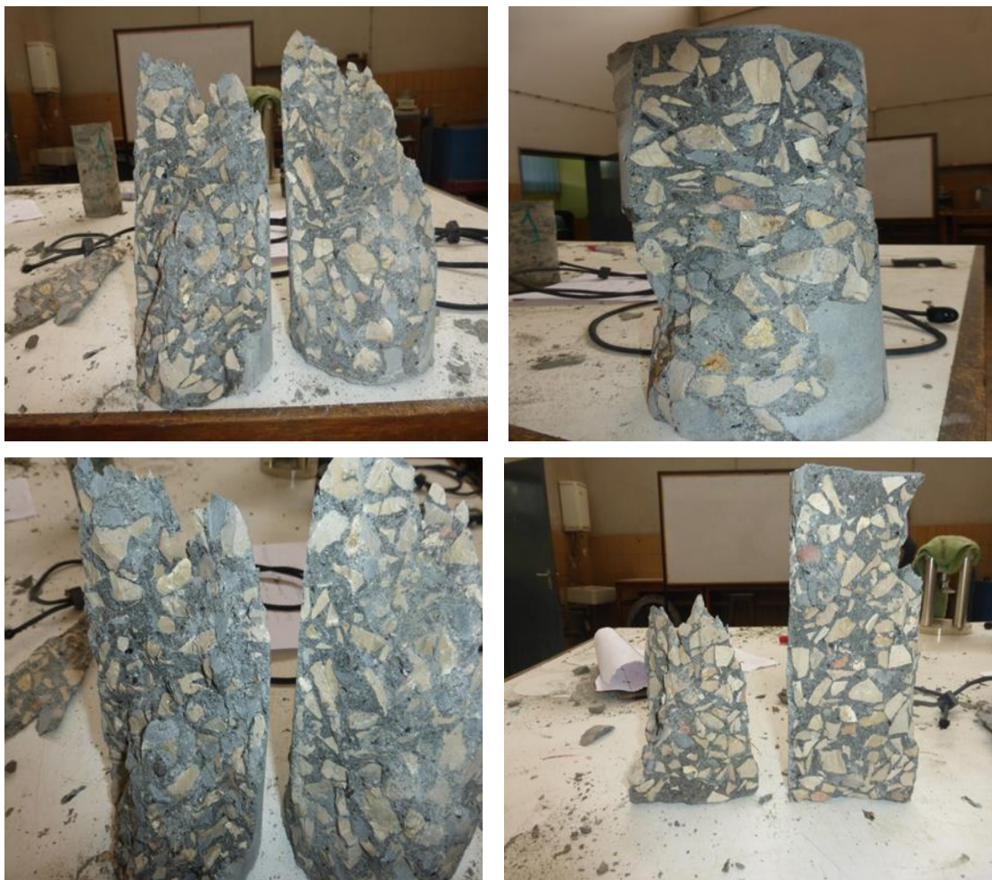
Figure 4-2 Fracture surface for concrete made using limestone based coarse aggregate
