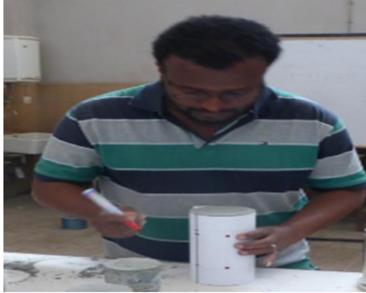
Figure 3-3 procedure for marking the points to which the transducers are to be attached
