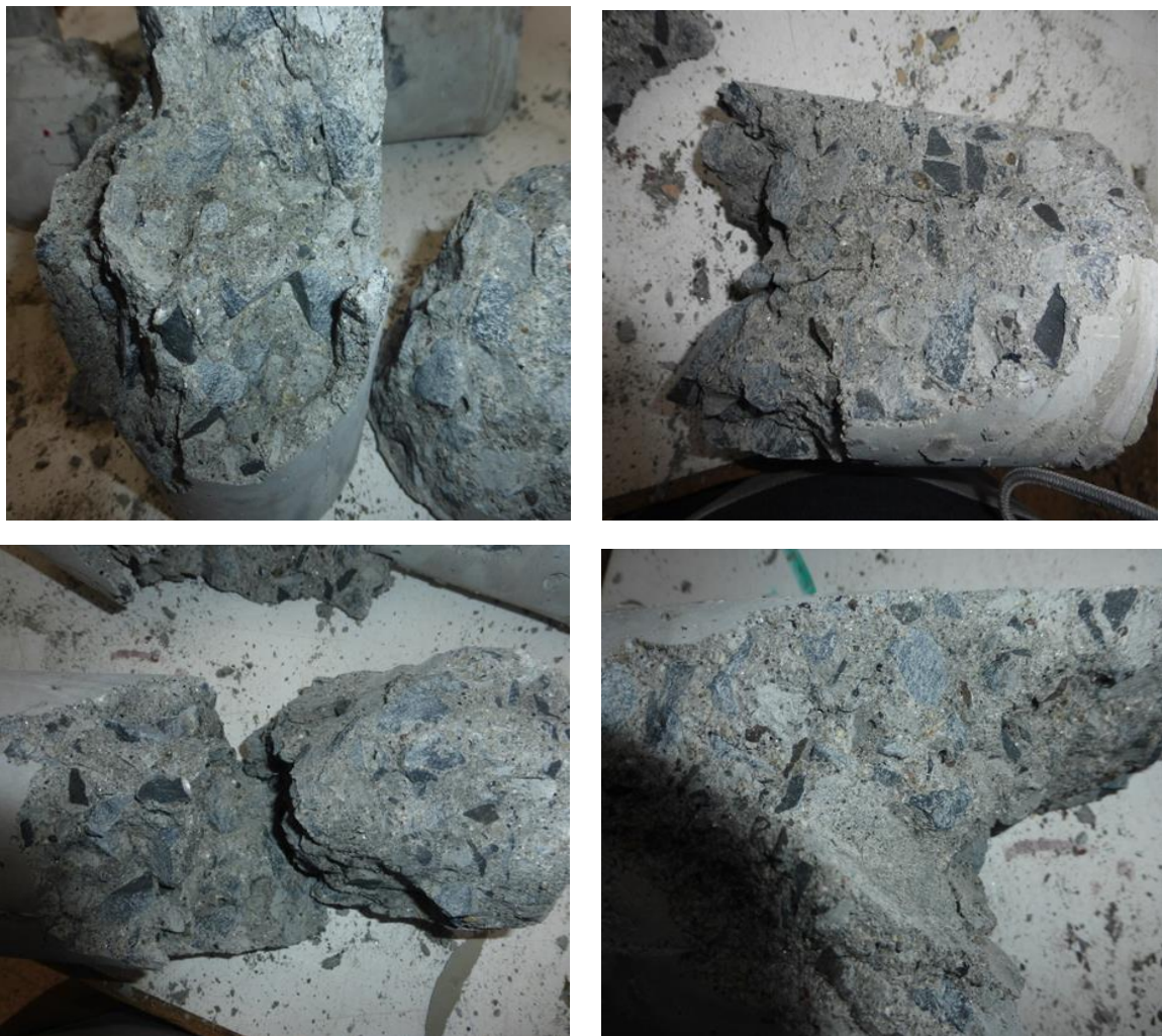
Figure 4-4 Fracture surface for concrete made using basaltic coarse aggregate
