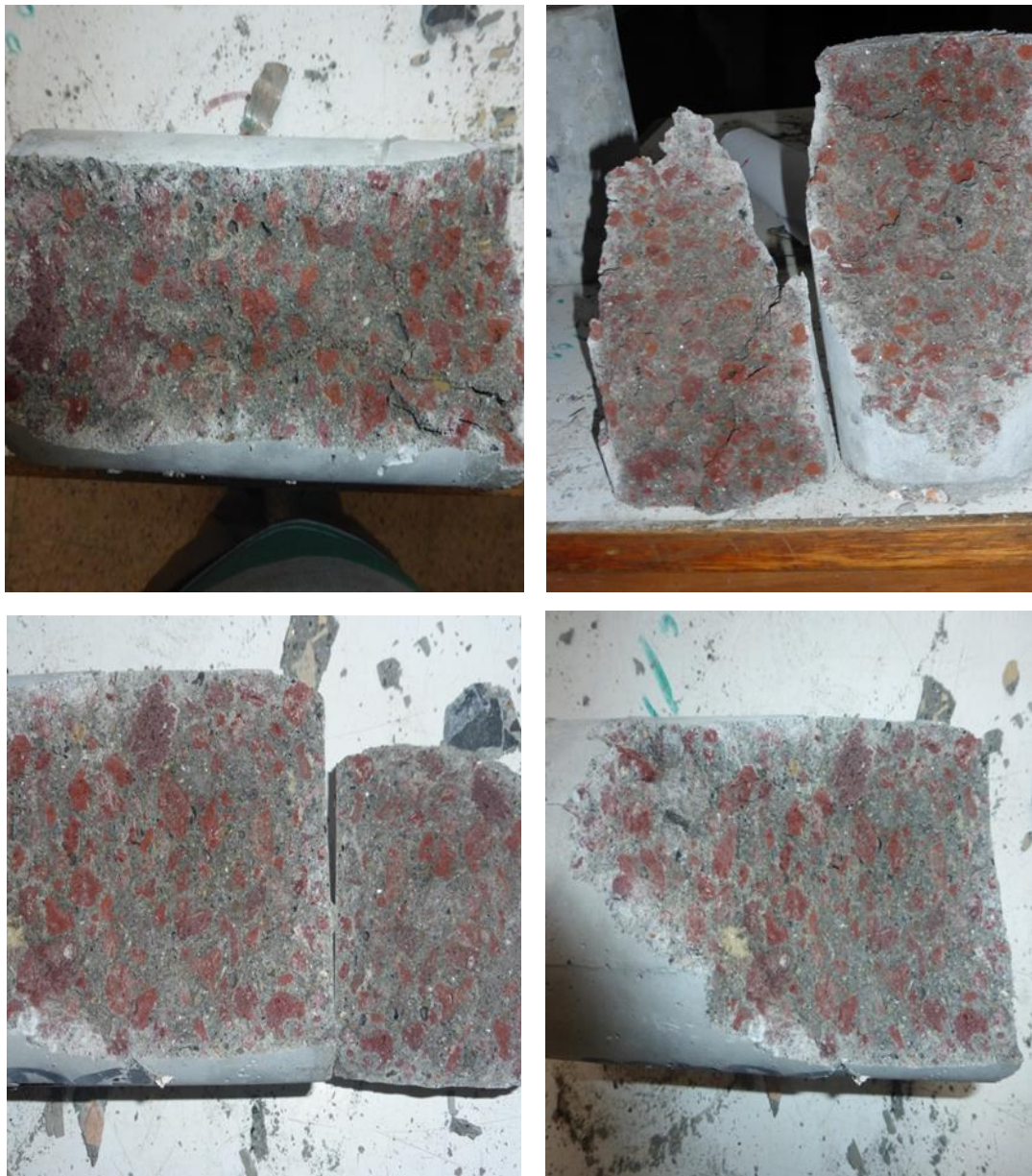
Figure 4-3 Fracture surface for concrete made using scoria based coarse aggregate
