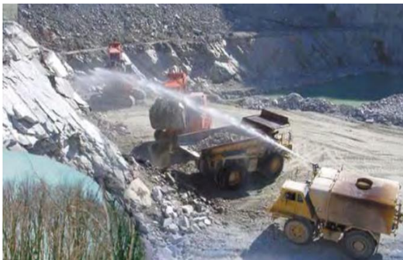
Figure 2.12 water trucks minimize dust in and around quarry (Langer, et al., 2001), as cited in (Semere, 2013)
