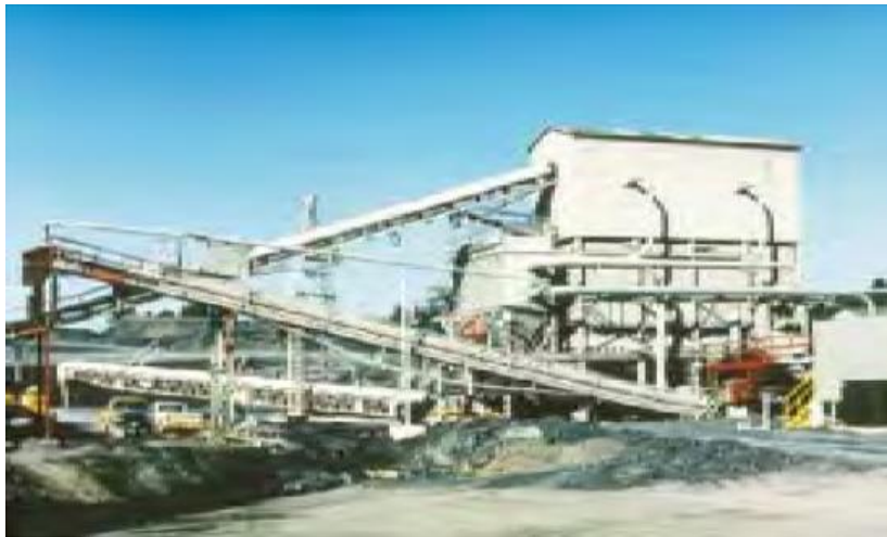
Figure 2.11 noisy equipment enclosed in sound-deadening structures (Langer, et al., 2001), as cited in (Semere, 2013)
