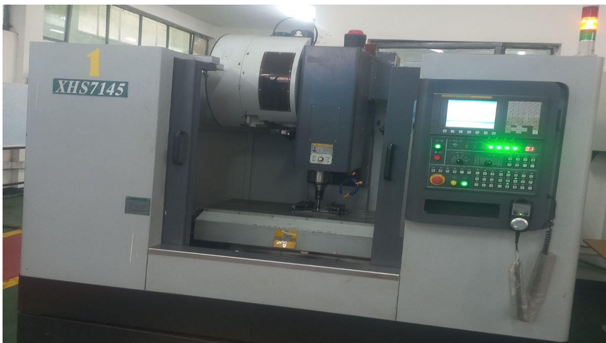
Figure 3.4 CNC milling machine with mounted fixture for FSW
