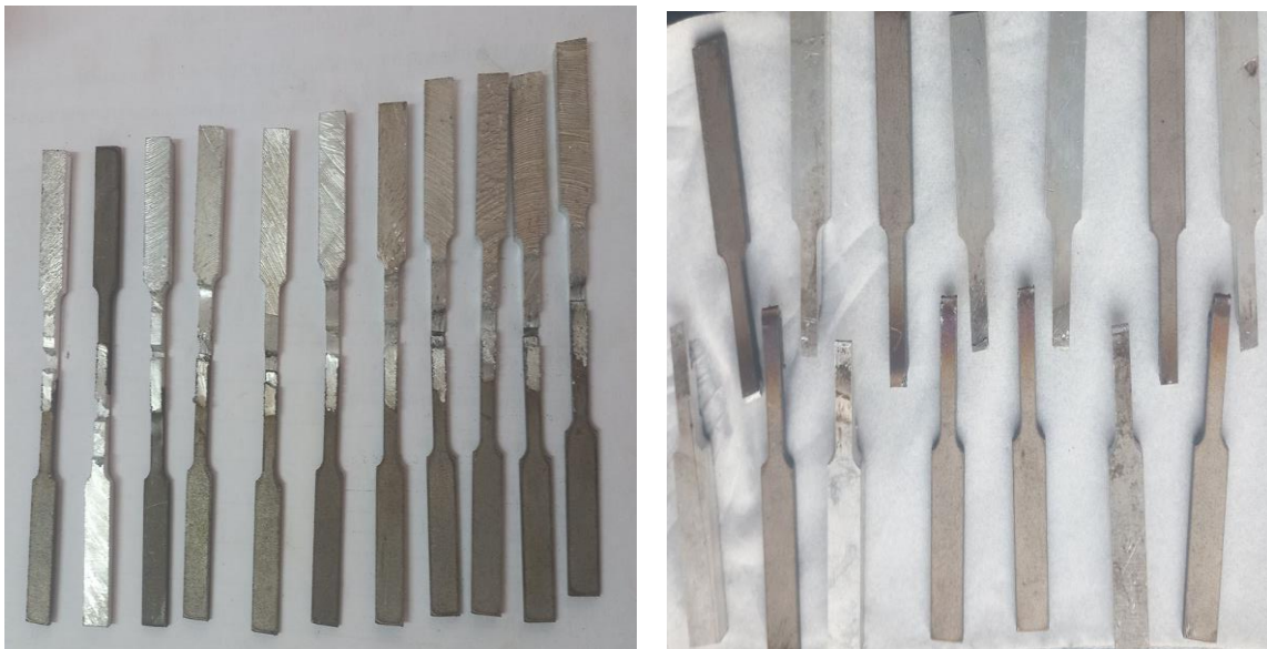
Figure 3.14: prepared tensile test specimen and after tensile test
