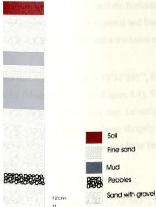
Figure 4.1 Section 1 taken from the Southwestern part of the catchment N 12°34'683'', E39°31'447'', (4.8 meters thick).
