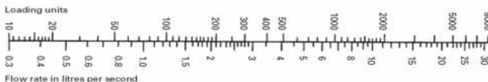
Figure 2 loading unit rate and fixture units
