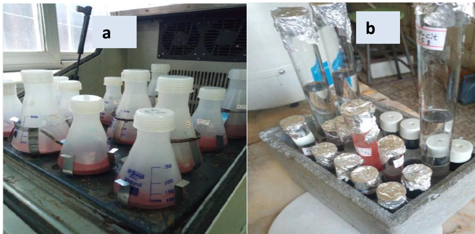
Figure 6. a) Adsorbent samples with Pb 2+ solution shaken in the rotary shaker. b) The remaining Pb 2+ ions concentration for AAS analysis.
