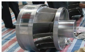
Figure 3-10: Horizontal Francis Hydro Turbine Generator [37]
