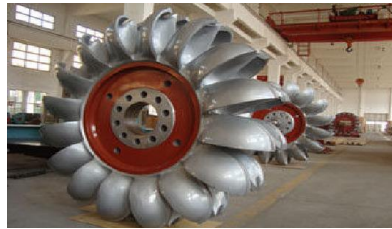
Figure 3-9: Pelton Hydro Power Turbine Generator, Multi type Turgo Turbine Unit [37]
