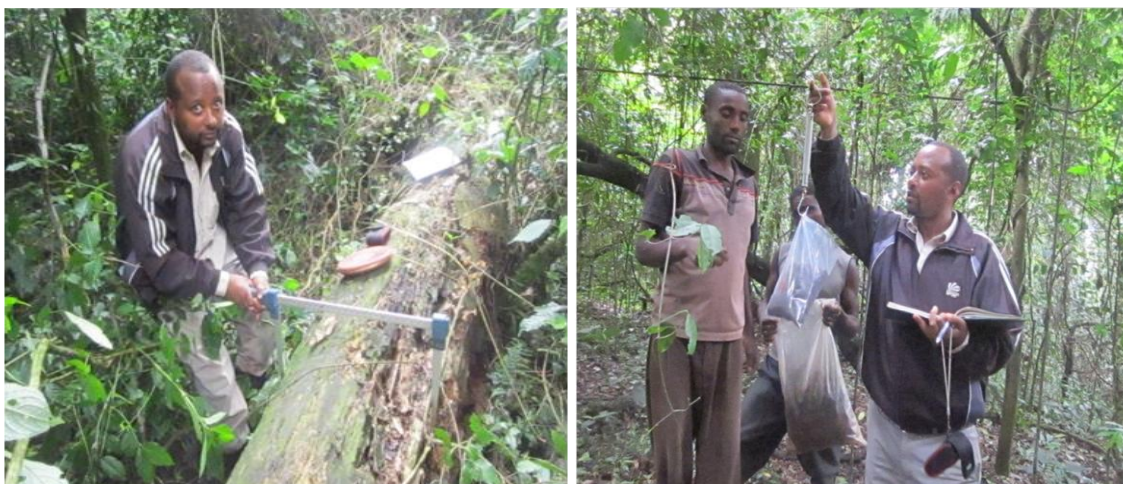
Appendix 15. Photos illustrating measurement for volume of a trunk and trimmed biomass
