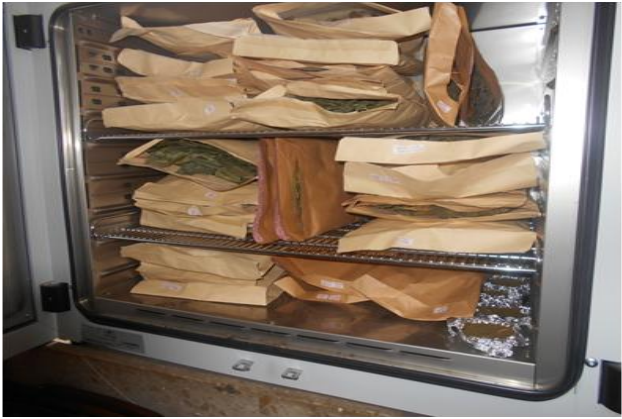
Appendix 16. Photos illustrating density measurement by water displacement and Oven drying leaf, wood, litter and herb samples biomass
