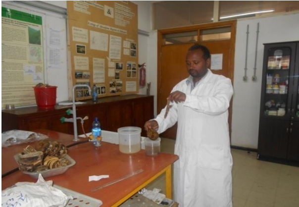
Appendix 16. Photos illustrating density measurement by water displacement and Oven drying leaf, wood, litter and herb samples biomass
