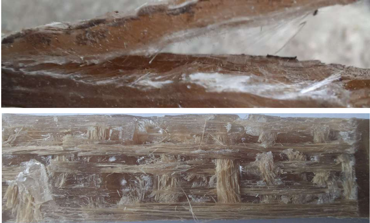
Figure 4-8 Pure Sisal reinforced composite after complete fracture
