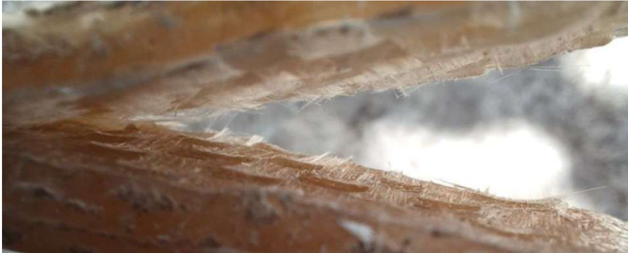
Figure 4-10 Hybrid composite after complete fracture
