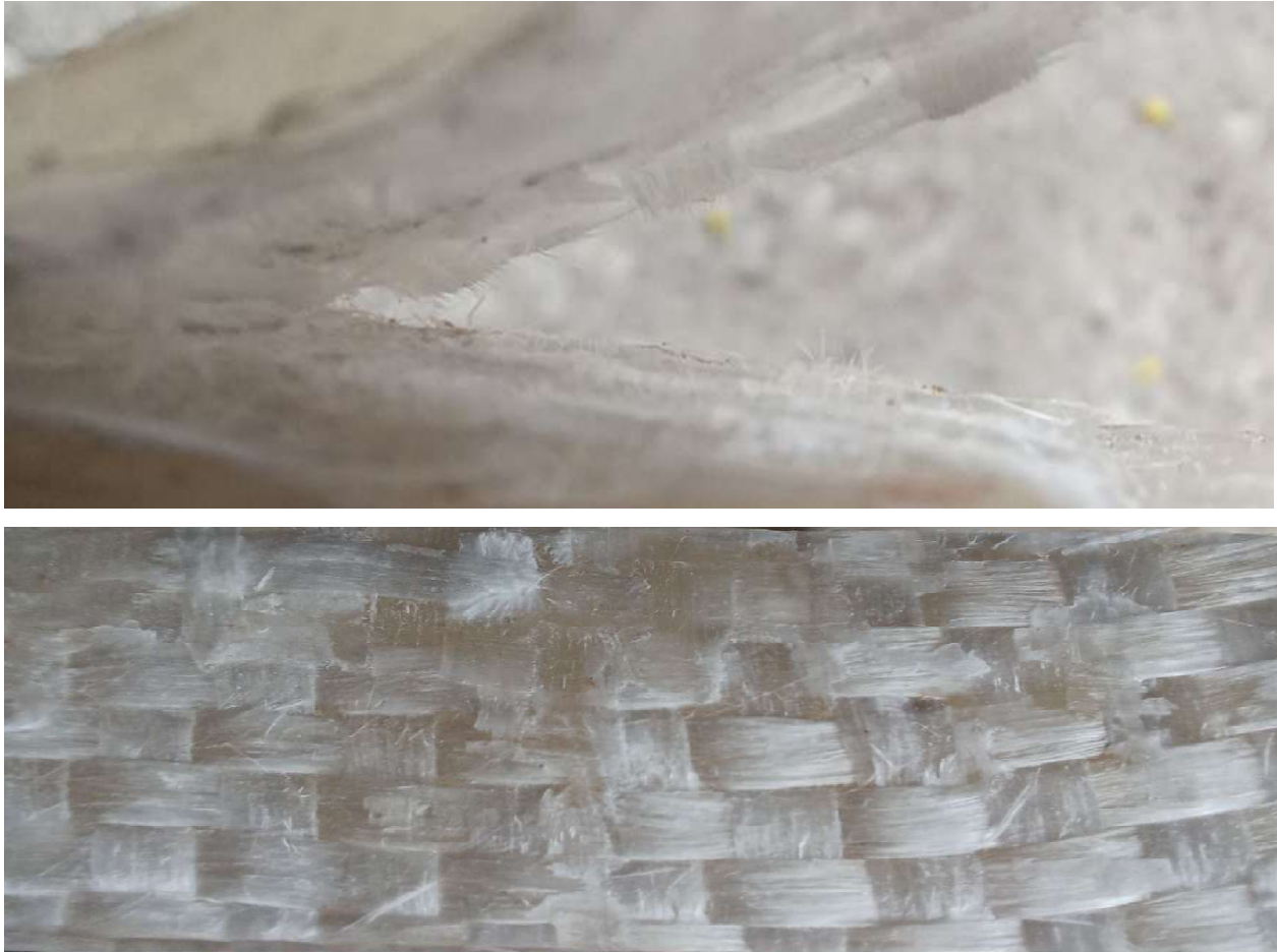
Figure 4-9 Pure glass fiber reinforced composite after complete fracture
