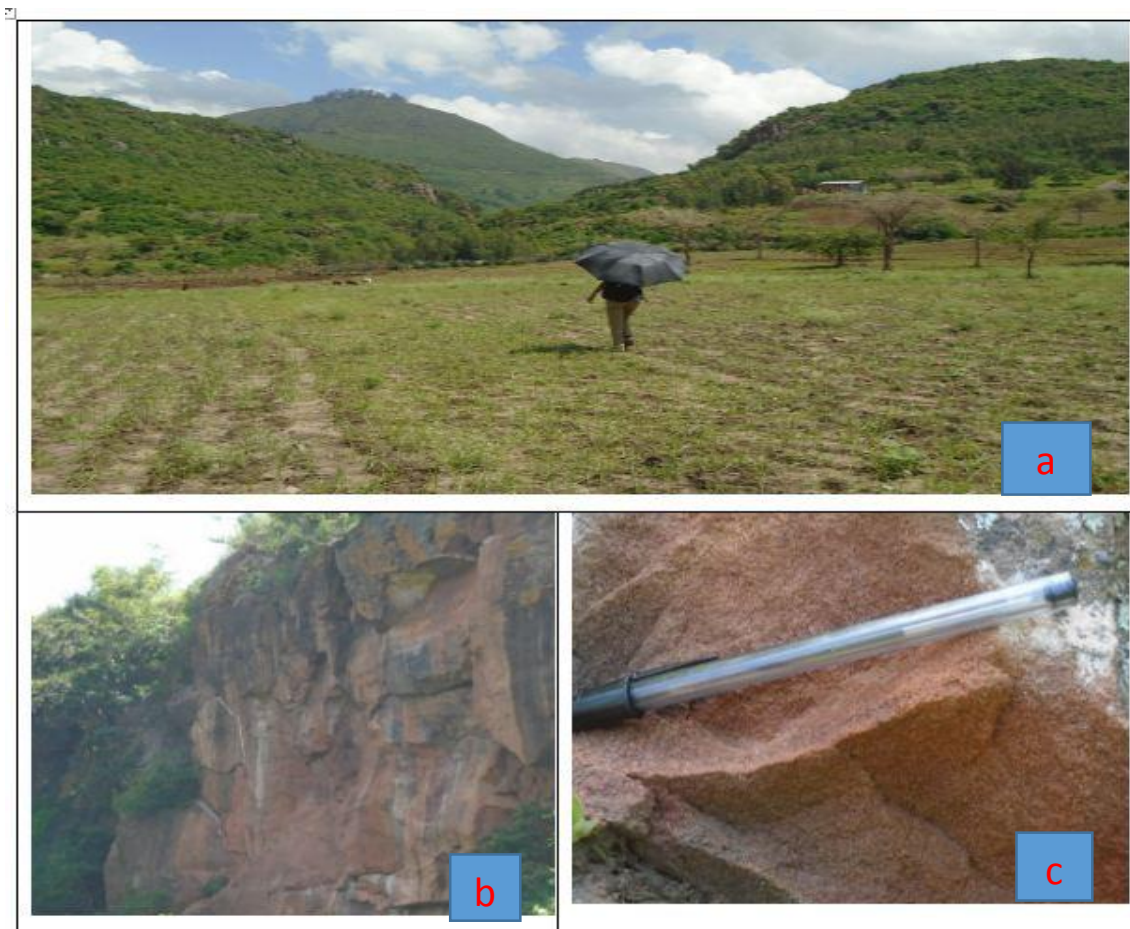
(a) the land forms of the sandstone rocks and the surrounding landscapes of Lebu SHP site (b) exposure of sand stone rock outcrop downstream of the proposed diversion weir site (c) Rock sample from the outcrop of the exposed sand stone rock at the propose diversion weir site.
