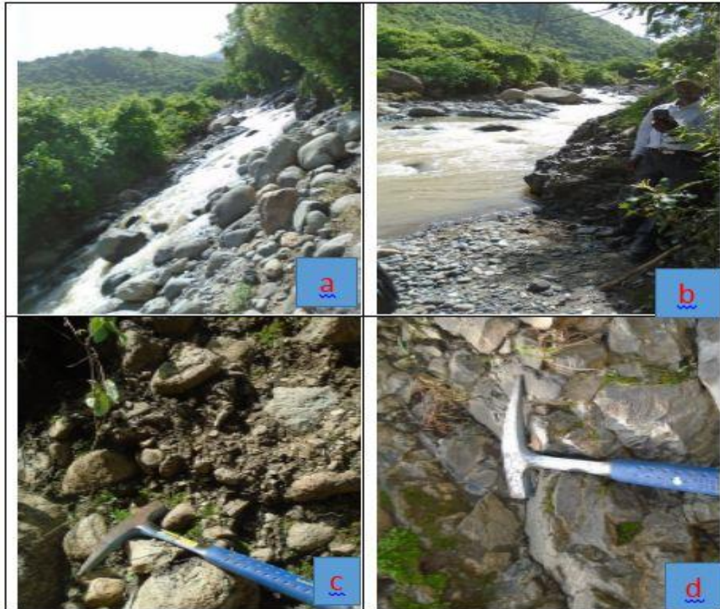
(a) shows the river section at the proposed diversion weir site of Weldia SHP, (b) shows the outcrop of basalt rock at the proposed diversion weir site of Weldia SHP site, (c) shows transported material deposit at the right bank of the river downstream of the proposed diversion weir site of Weldia SHP site and (d) shows joints on outcrop of basalt rock at the proposed diversion weir site of Weldia SHP site,
