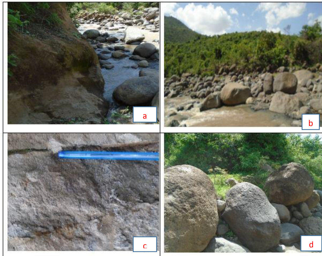
(a) shows out crop of welded pyroclastic rocks at Rufael SHP diversion weir site the left bank of the river, (b) shows rock exposure at the right bank of the river the proposed diversion weir of Rufael SHP site (c) rock sample of the out crop of slightly weathered welded pyroclastic rocks at Rufael SHP diversion weir site and (d) shows the bolder rocks at the site of proposed diversion weir of Rufael SHP.
