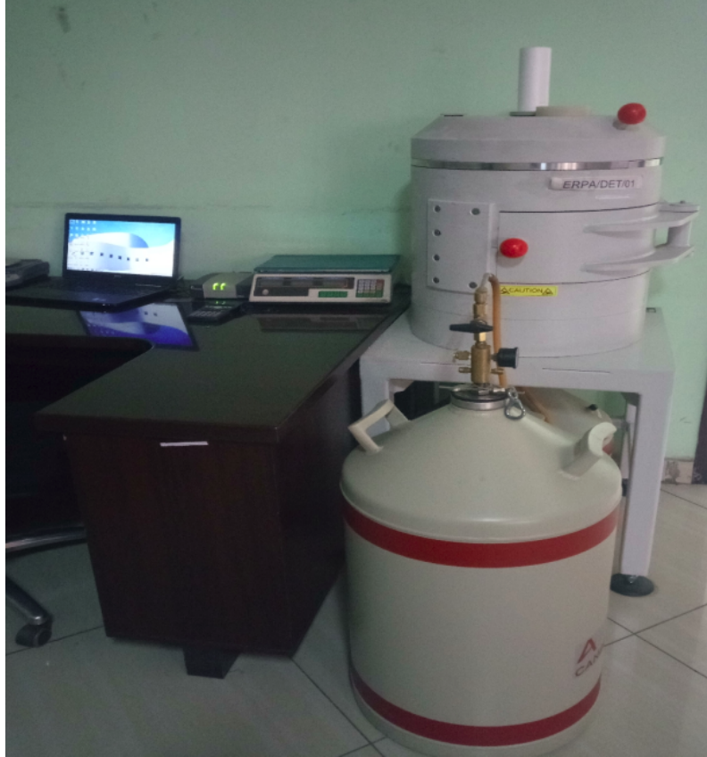
Figure 3.2: Gamma spectrometry mounted with HPGe detector and DSA circuit (ERPA-Laboratory)
