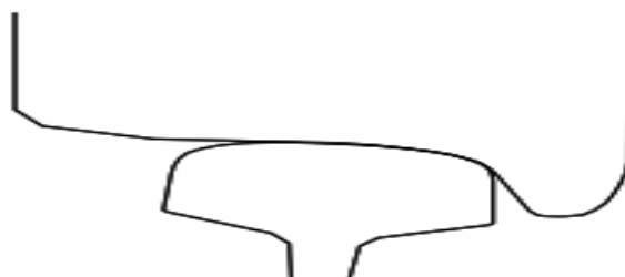
Figure 3. 1 Conformal contact (between the gauge corners of the rail with the wheel throat) [4]
