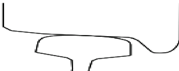
Figure 3. 2 Non-conformal contact (between wheel tread and rail head) [4]
