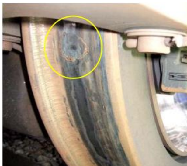
Figure 1. 2 a wheel flat formed by wheel-rail slip in the contact [22]
