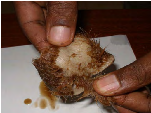
Fig 8. Results of cow hide dehairing experiment: (1) raw hide before dehairing, (2) control, (3) enzyme treated cow hide dehairing with fingers, (4) dehaired hide after few hours showing removal of scud and presence of natural hide pore on surface.
