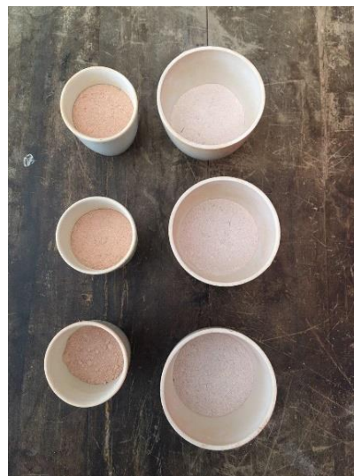
Figure 5-12: Kaolin samples before heating (Red on the left and White on the right)
