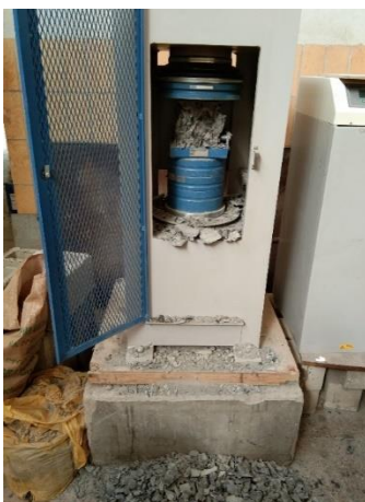
Figure 3-9: Crushing concrete cubes using a compression machine and its result
