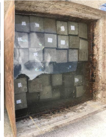
Figure 4-3: Curing of concrete cube samples
