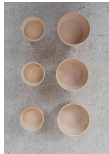
Figure 5-13: Kaolin samples after heating (Red on the left and White on the right)
