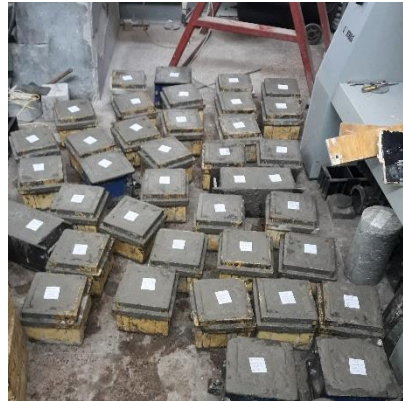
Figure 4-1: Concrete placed in 15cm cube molds
