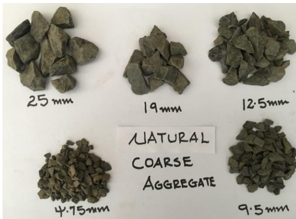
Figure 3-5: NCA retained on the specified sieve sizes
