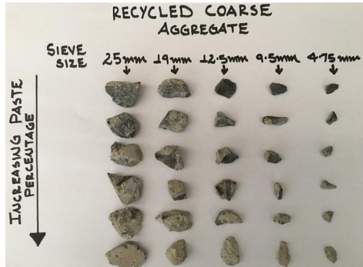
Figure 3-11: RCA with increasing paste percentage
