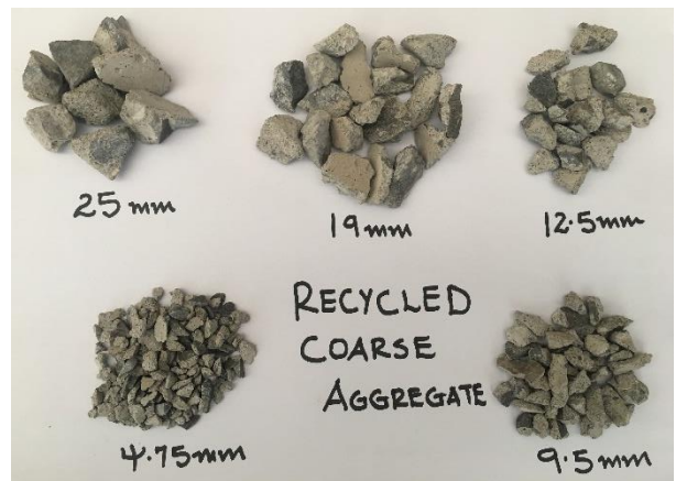
Figure 3-6: RCA retained on the specified sieve sizes
