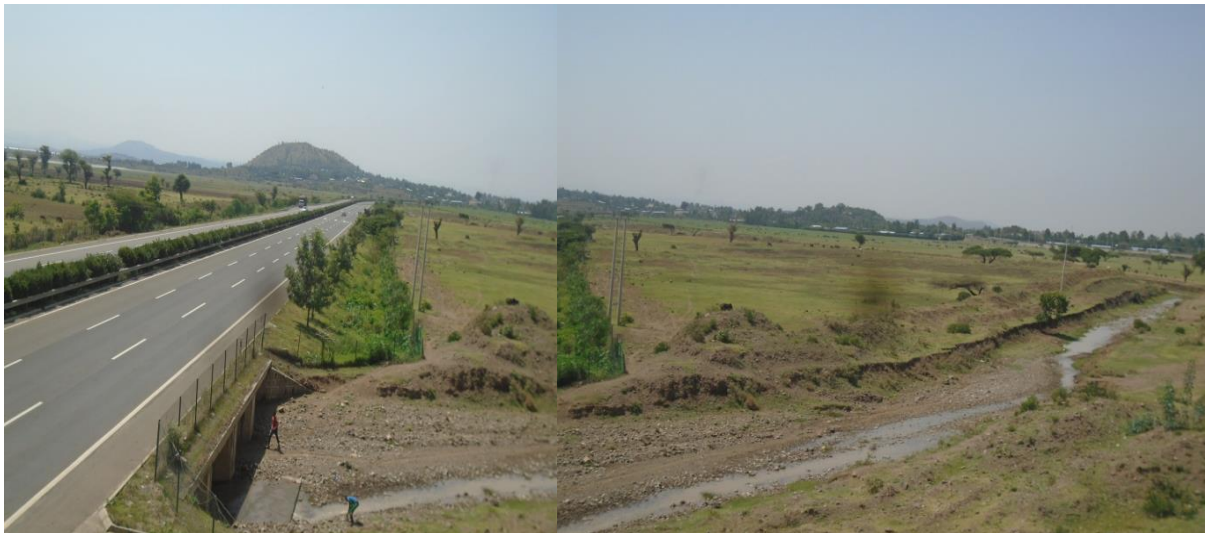
Picture 4. Diverted water flow of (iyyitu) river due to (Addis-Adama) high way construction.
