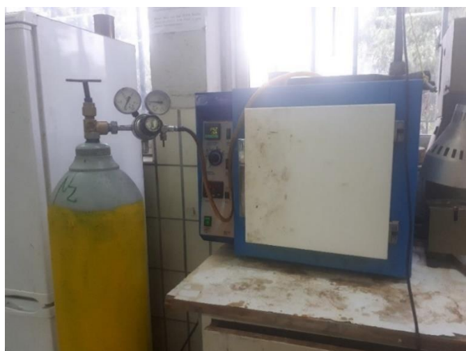
Figure 3-5 . Sulfonation of activated carbon under nitrogen gas
