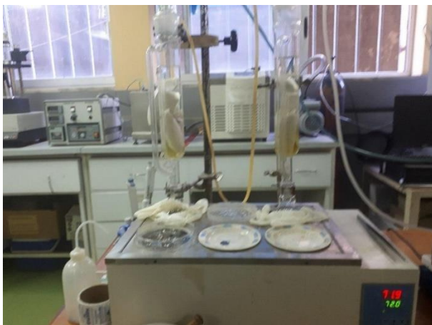
Figure 3-10. Soxhlet extraction of podo carpus falcatus seed oil
