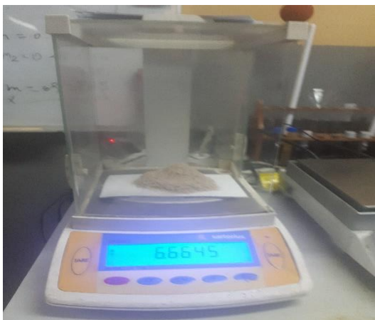
Figure D-1 Measuring Balance of crashed seed for Soxhlet and extraction unit with water bath
