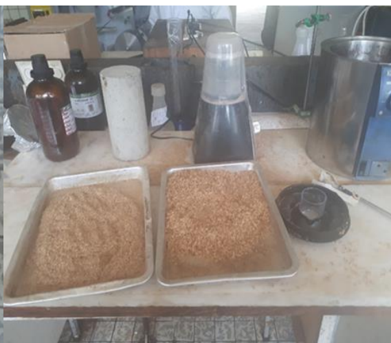
Size reduction of rice husk by juice blender (b)
