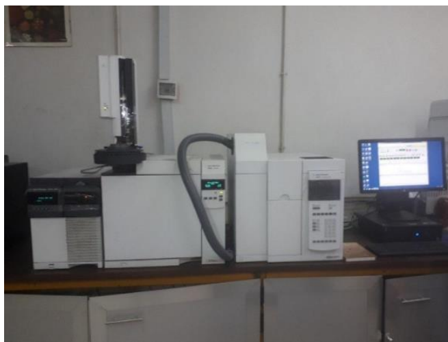
Figure 3-14. Gas Chromatography Mass Spectroscopy (GC/MS) analyzer of podo carpus falcatus seed oil
