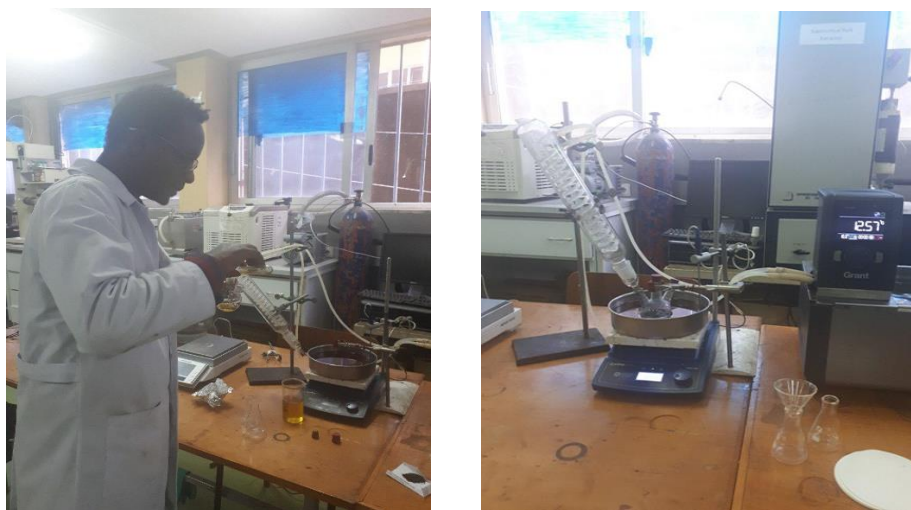
Figure 3-16. Preparation of sample for each run(a) and experimental setup of epoxidation reaction(b)
