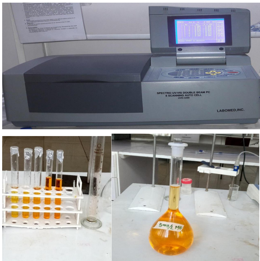
Figure 3-7. UV -spectroscopy and methyl orange solution preparation
