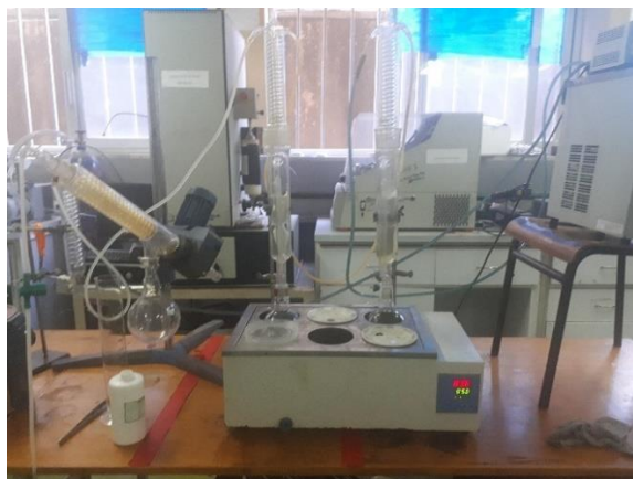
Figure D-1 Measuring Balance of crashed seed for Soxhlet and extraction unit with water bath
