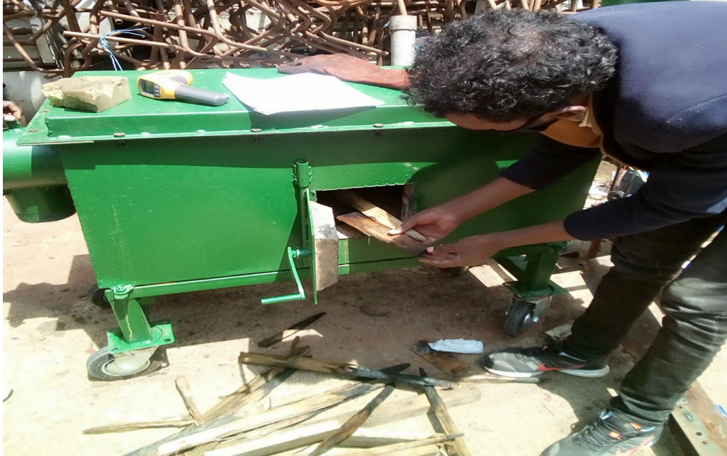
Figure 3-5 inserting the wood into the combustion chamber
