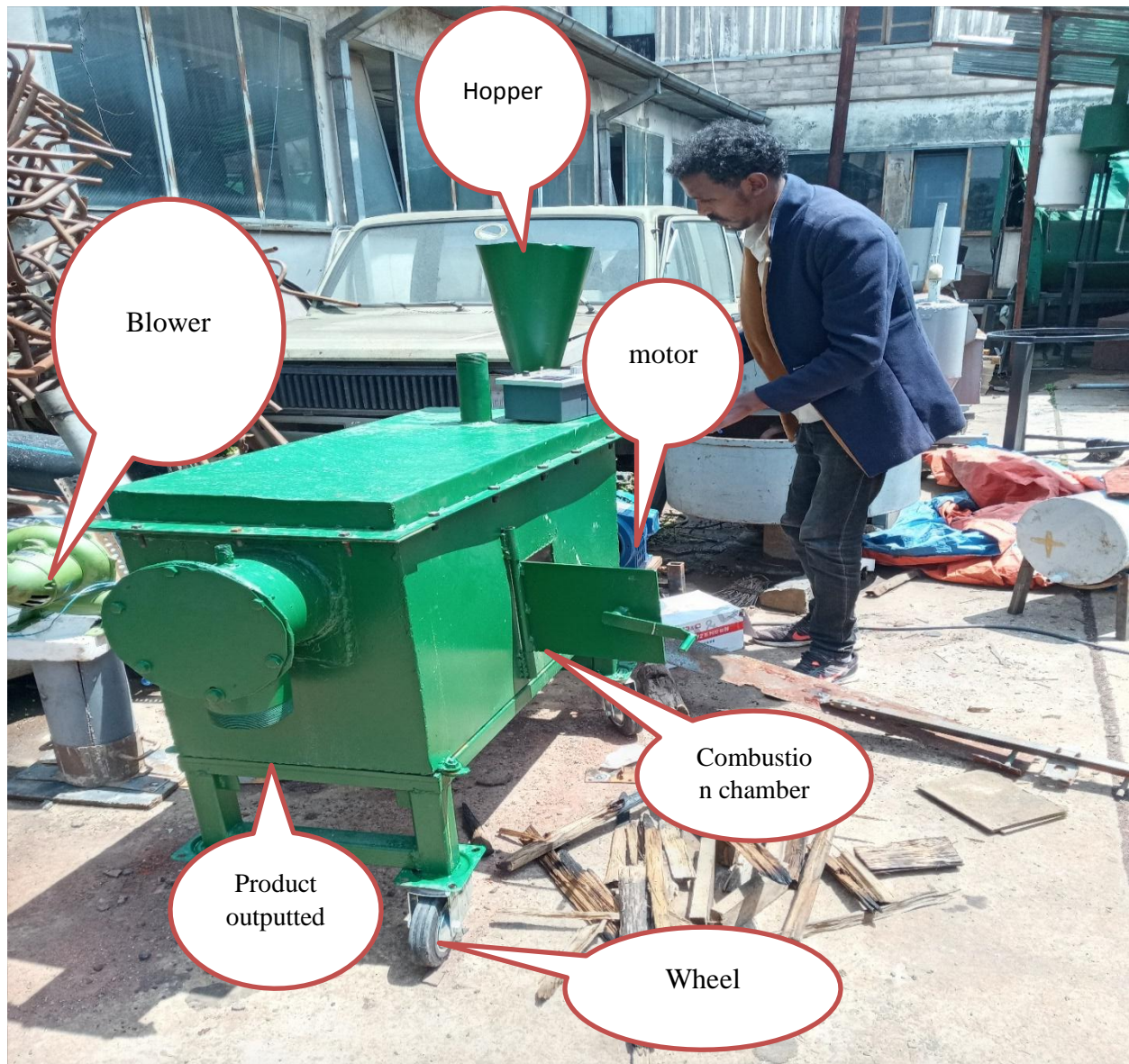
Figure 4-2 Prototype of the developed continuous biochar producing machine
