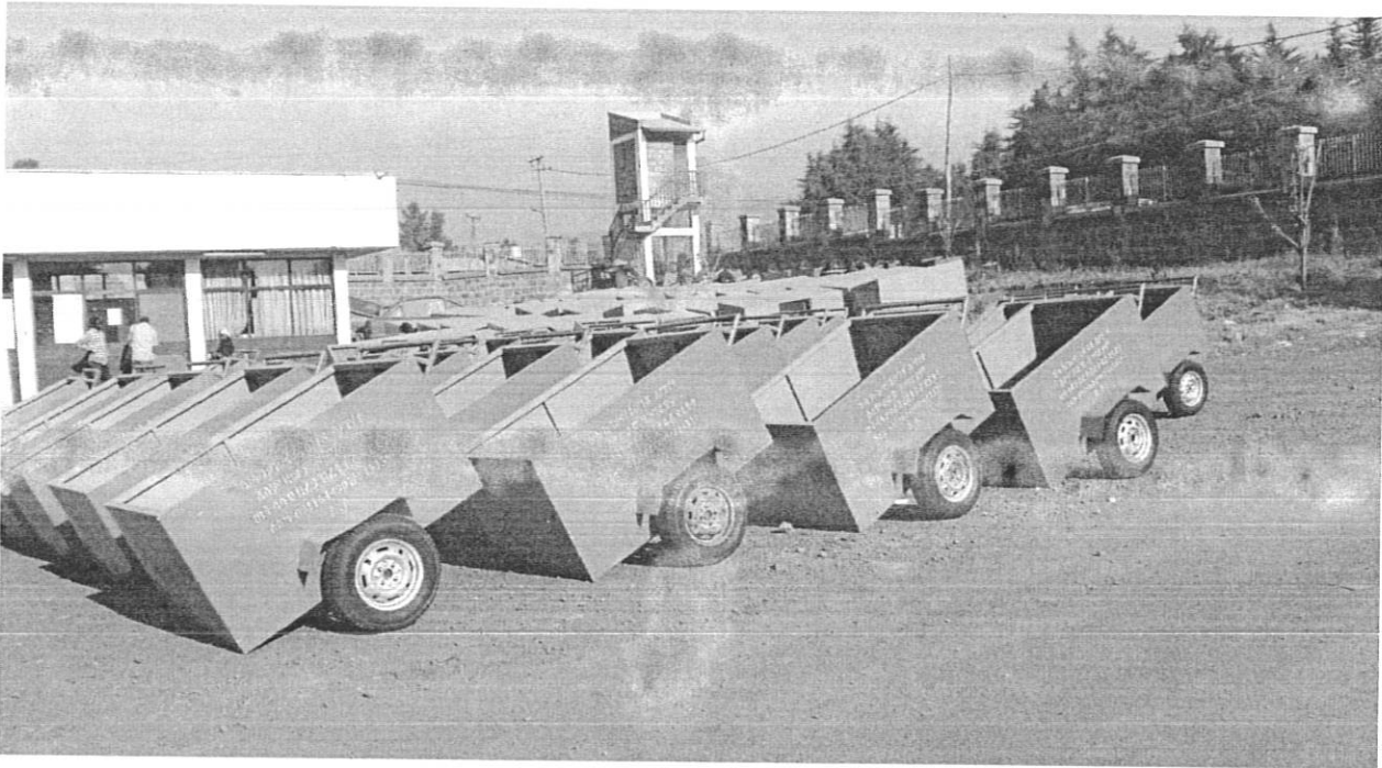
A two legged wheeled container being used for transporting solid wastes by micro sanitary enterprises
