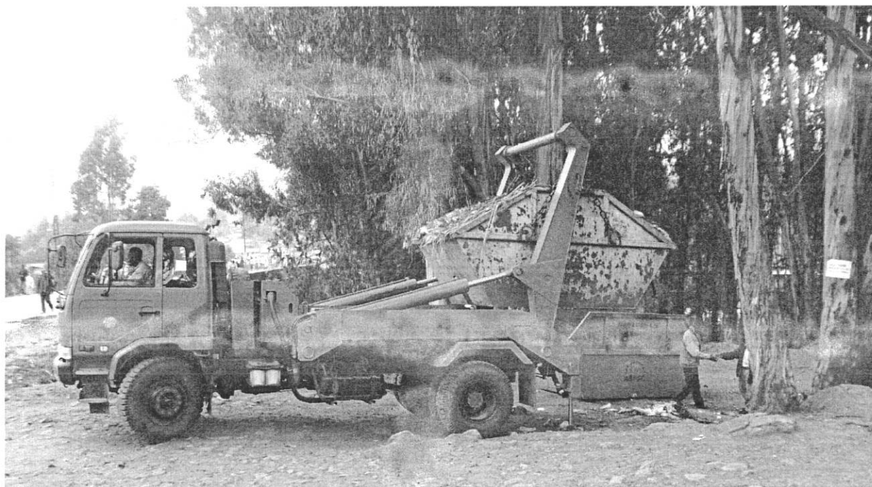
A dumpster carrying truck replacing a filled container with an empty one
