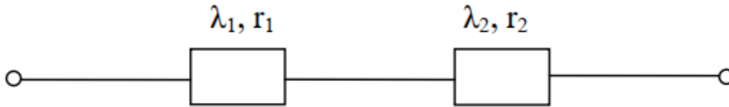
Figure 2- 3 Series Structure (System) For Two Components
