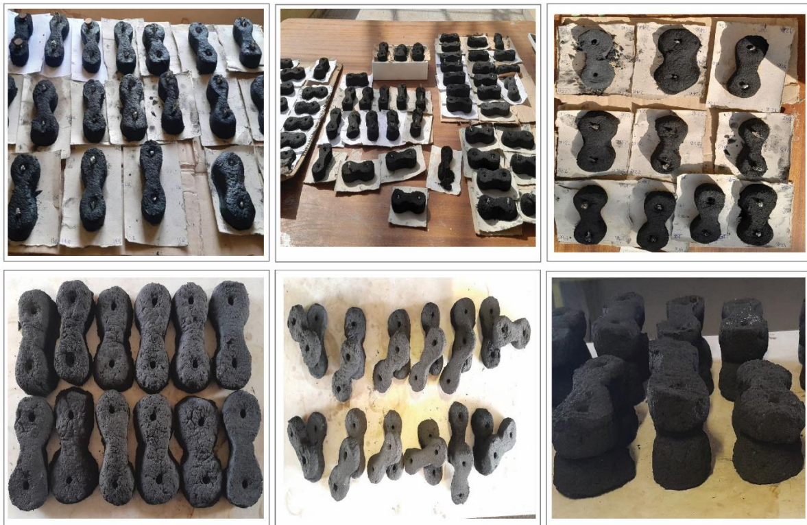
Figure 6. Biomass briquette with the composition of avocado, bagasse, and banana peel
