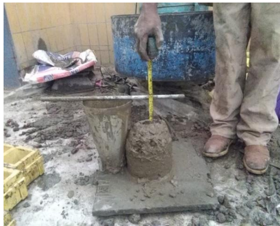
Figure 3. 14 Slump cone and slump measurement of fresh concrete mix
