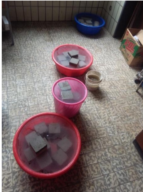
Figure 3. 8 Concrete samples in curing baths
