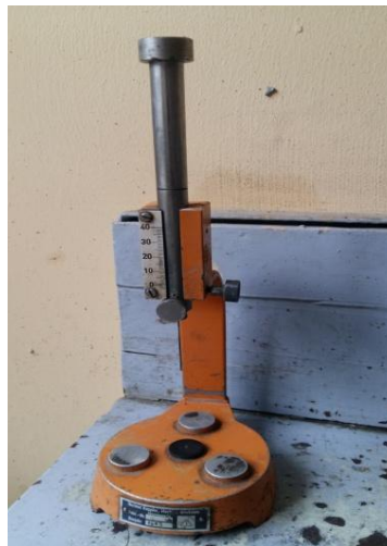
Figure 3. 13 Viccat apparatus for testing consistency and setting time
