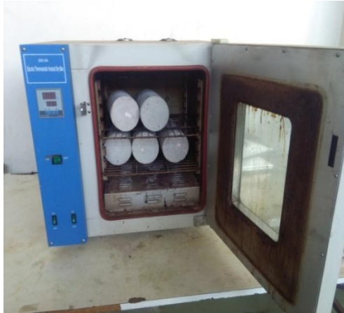
Figure 3. 17 Oven to dry sample for water absorption test
