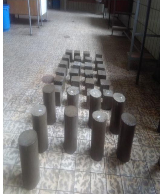
Figure 3. 7 concrete surfaces drying and ready for crushing
