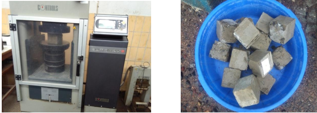
Figure 3. 15 Compressive strength measuring machine and some of the crushed samples
