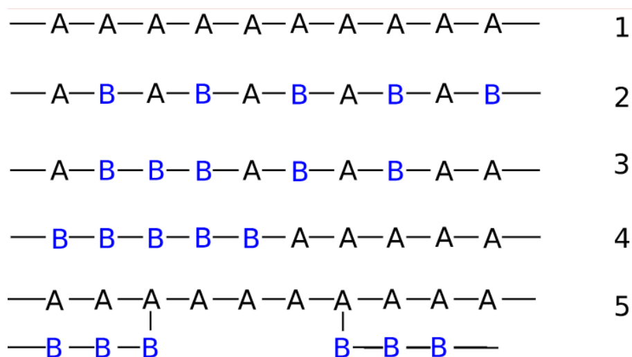
Figure 2.1: Different types of polymers: 1) homopolymer 2) alternating copolymer 3) random copolymer 4) block copolymer 5) graft copolymer. This diagram is taken from Wikipedia
