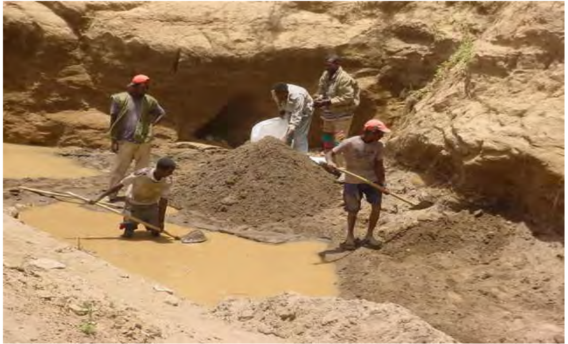
Fig: 2.4 Traditional way of sand production in Ethiopia [3]
