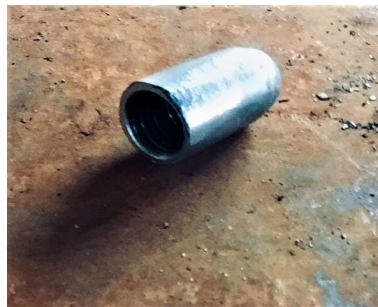
Figure 3.43: Modeled interchangeable hemispherical tup
