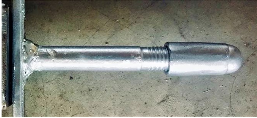
Figure 3.42: Actual Prototype of striker assembly
