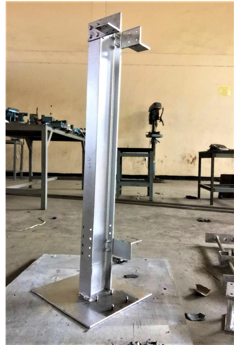
Figure 4.2: Drop tower with foundation
