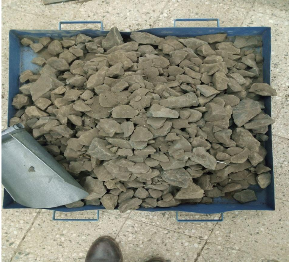
Figure 15: Fouled ballast sample
