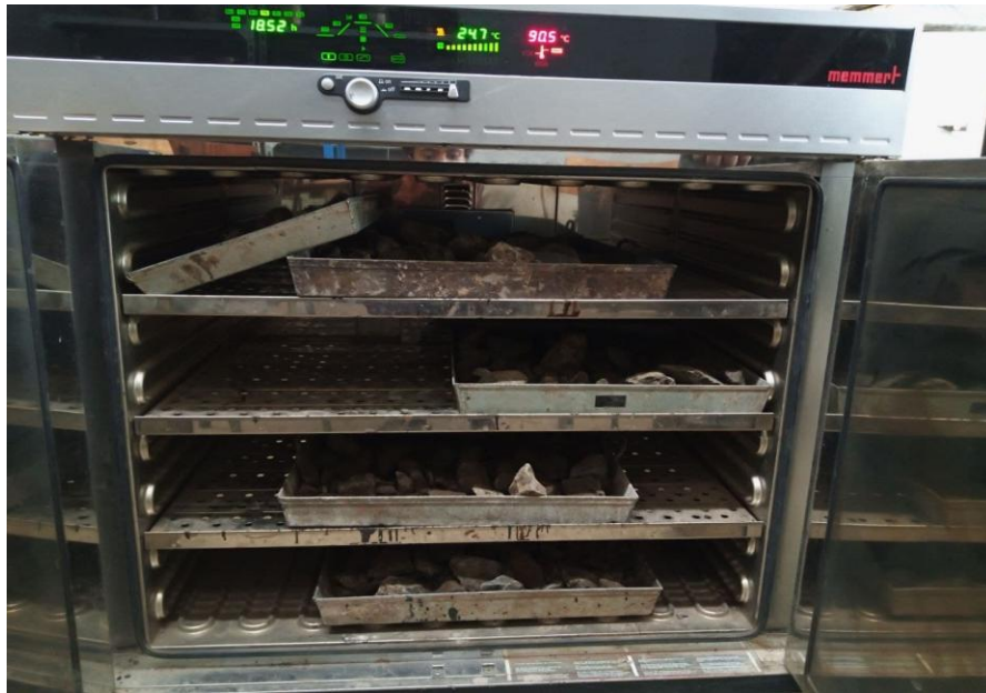
Figure 16: Oven for drying aggregate sample
